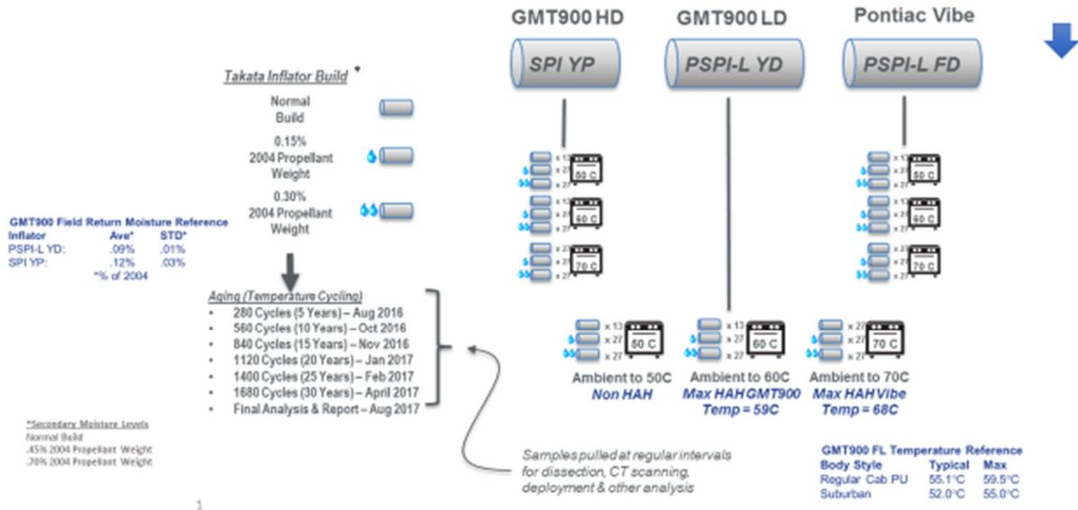
**Figure 2: Test design for OATK Accelerated Aging Study (provided by GM)<sup>87</sup>**
