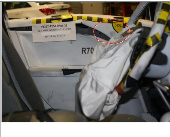
Figure 11. Head contact with door panel in PCb RMBDtV test
