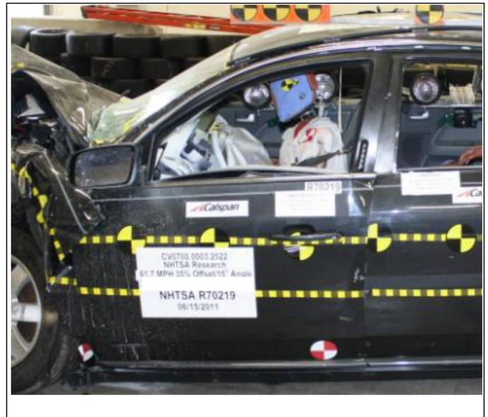
Figure 13. Door frame deformation in PCb RMBDtV test
