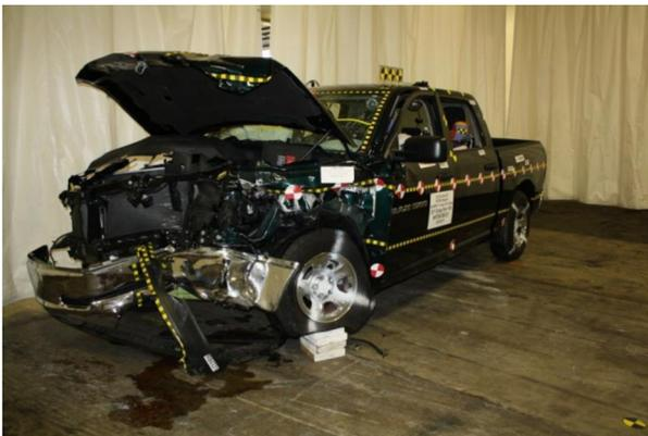
Figure 32. PU1 oblique exterior crush
