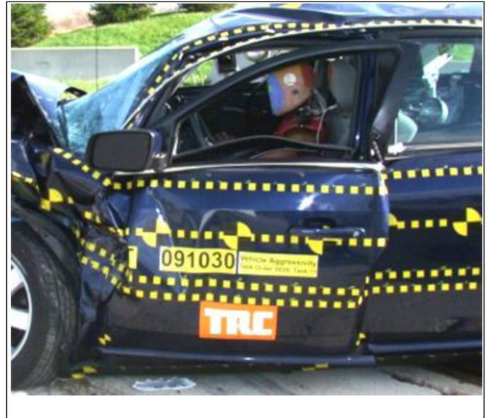
Figure 12. Door frame deformation in PCb ViV test
