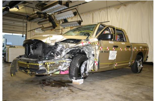
Figure 33. PU1 SOI exterior crush
