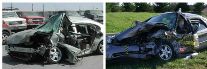
**Figure 25. Non-Fatal Oblique Case Comparison. Left picture is the CIREN case and right picture is PCa**
