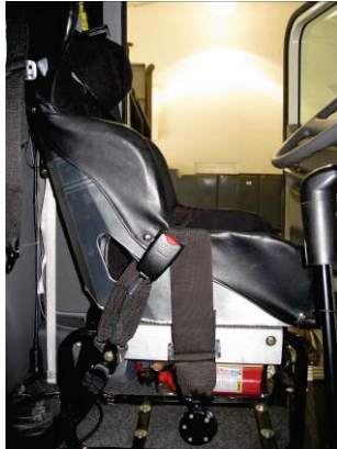
AP Figure 6. Driver restraint system.
