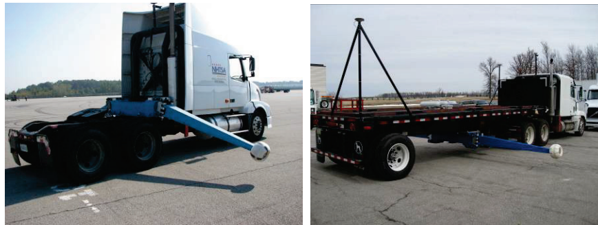
AP Figure 1. Tractor and trailer mounted outriggers.
