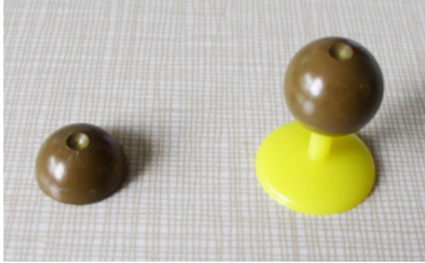
Figure A2. Sphere and hemisphere targets with divot for probe digitizing.
