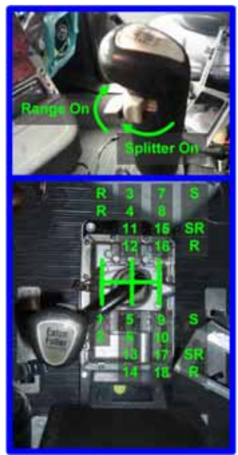
Figure 2.6 - Truck cab shifting
