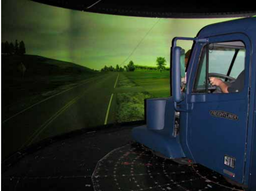
Figure 2.3 - Truck cab in the NADS dome
