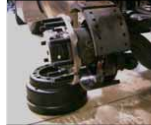
Drive Axle: Standard S-Cam Drum Brake
