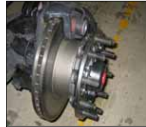
Steer Axle: Vented Air Disc Brake
