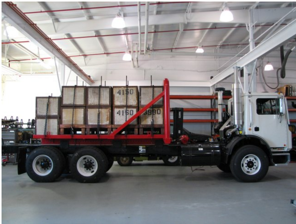
Figure 2.1. Mack MR-688-S Chassis-Cab Truck Loaded to GVWR With Concrete Blocks to Simulate a McNeilus Refuse Hauler
