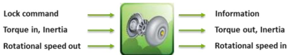
**Figure 6-9 - Autonomie Torque Converter Model Input/Output**
