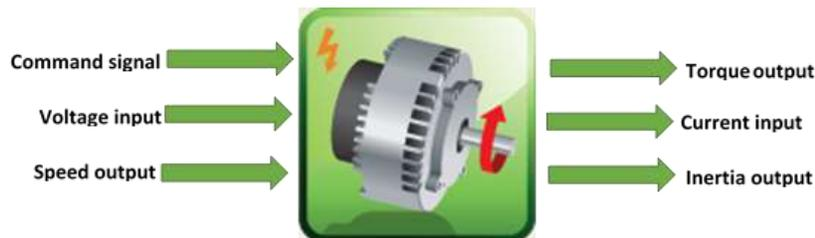
Figure 6-12 - Autonomie Electric Machine Model Input/Output
