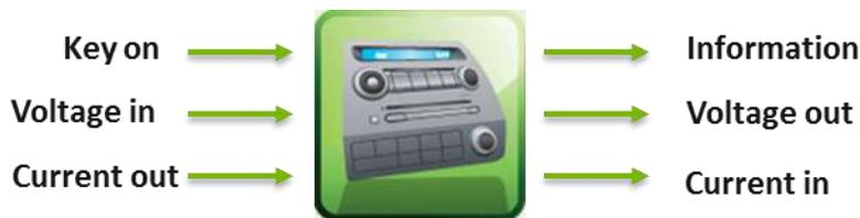
**Figure 6-14 - Autonomie Electrical Accessories Model**
