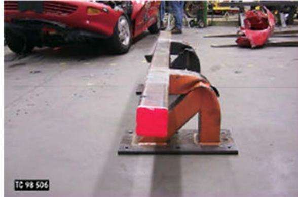
**Figure F-2 Crash test, Chevrolet Cavalier into 480 mm guard at 65 km/h. Note the highly deformed guard**
