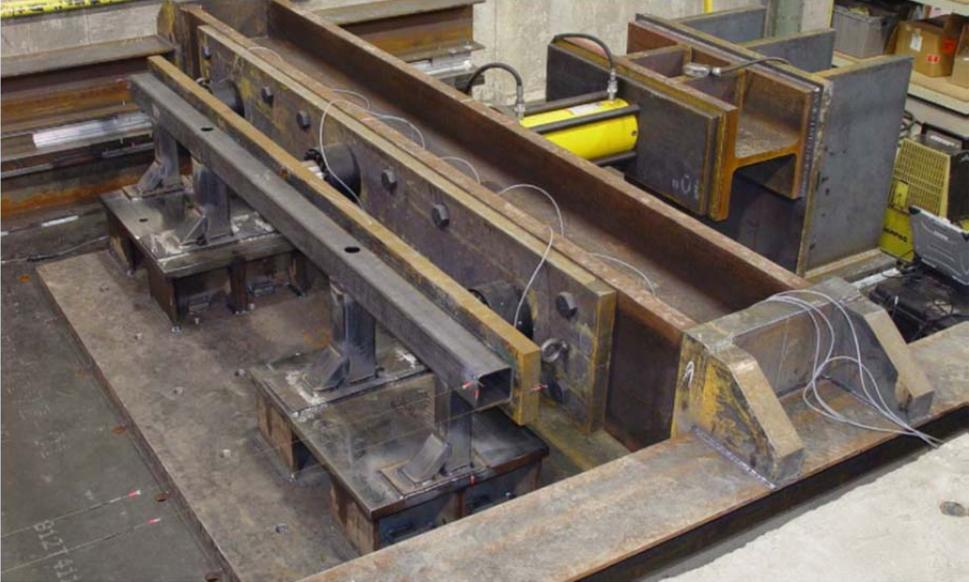
Figure F-4 View of test rig developed for uniform load application
