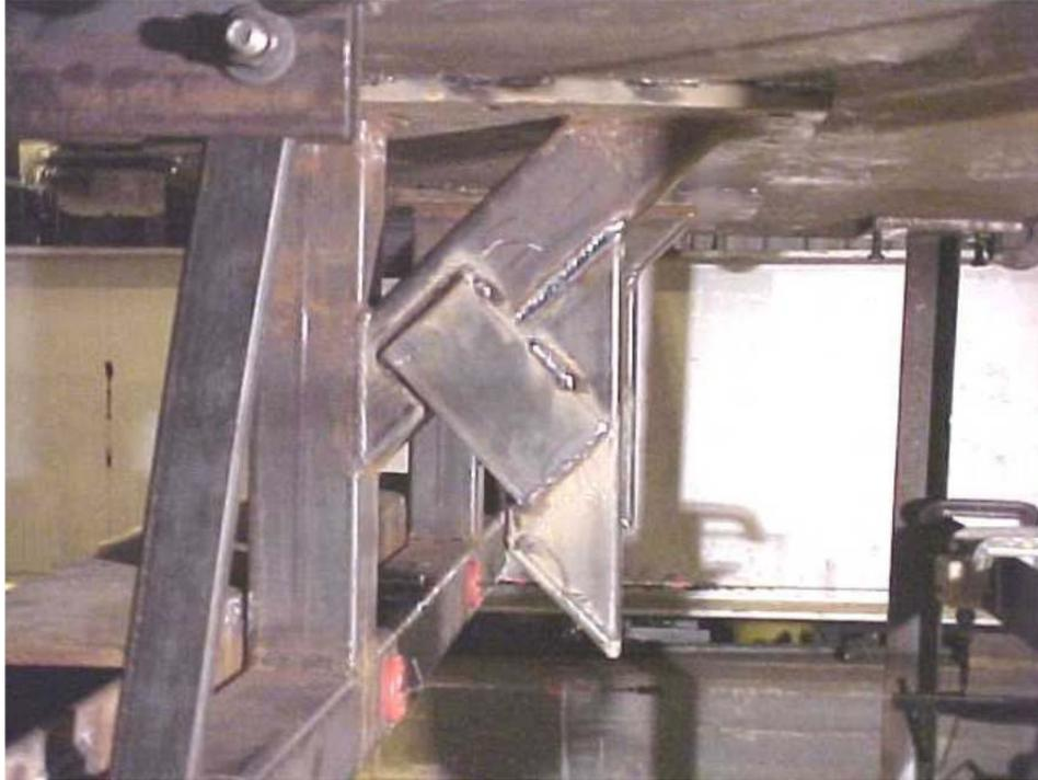
**Figure F-5 View of displacement stop feature used to minimize vertical travel of horizontal member.**
