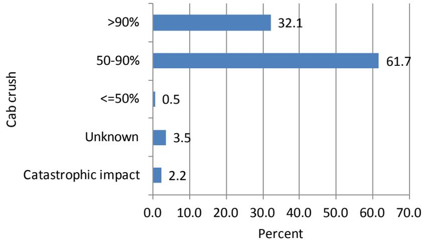
**Figure 26 Distribution of Cab Space Remaining, Truck Rollover and Subsequent Contact**
