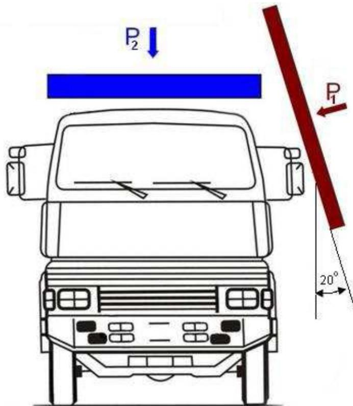
Figure 9 Roof strength test (Test C)
