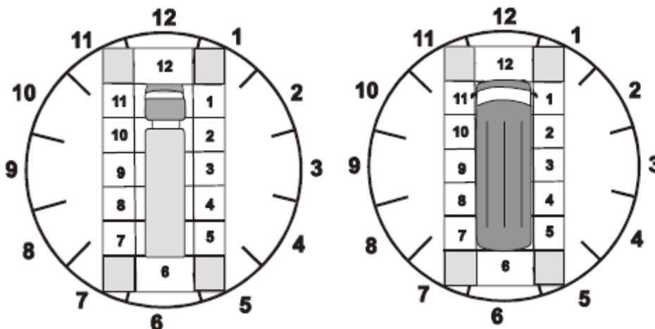
Figure 12 Schematics Used to Code Impact Point on Trucks in FARS
