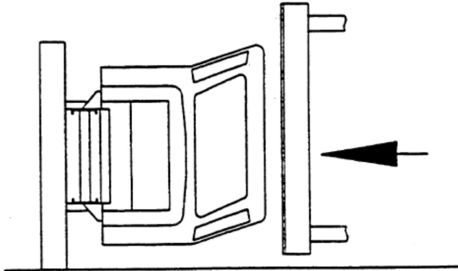
**Figure 6 Quasi-Static Roof Load Configuration**
