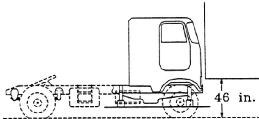
**Figure 4 Vertical Position of Platen Contact**
