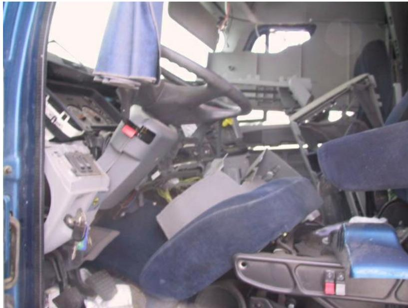
**Figure 36 Cab Interior Showing Damaged Seat and Instrument Panel Intrusion**
