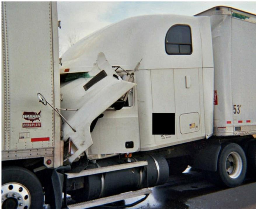
**Figure 28 Rear Hood Intrusion into Drivers Compartment**
