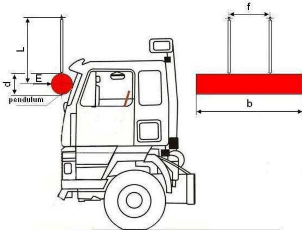
Figure 8 Front pillar impact test (Test B)
