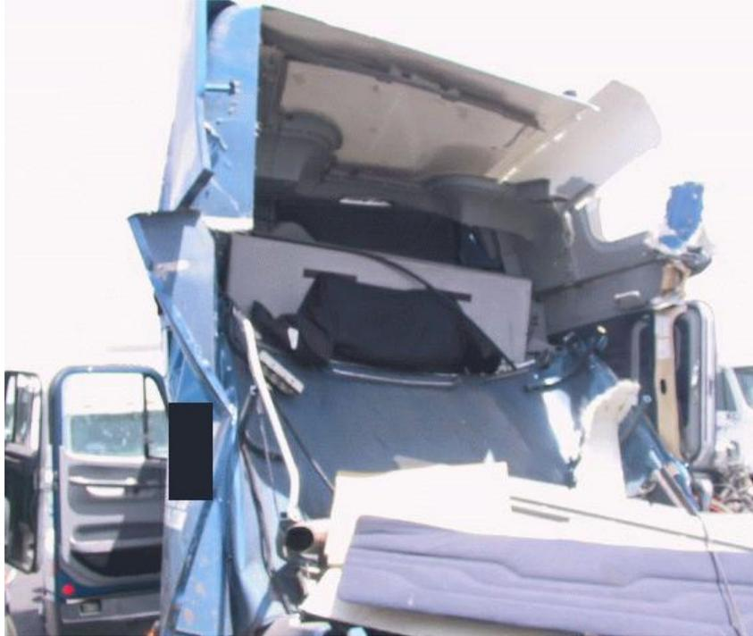
**Figure 33 Rear Intrusion from Trailer in Frontal Impact**
