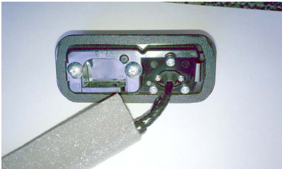
Figure 25 – Camera removed from vehicle showing OEM compressible water-tight foam seal on perimeter which would be against vehicle body.
