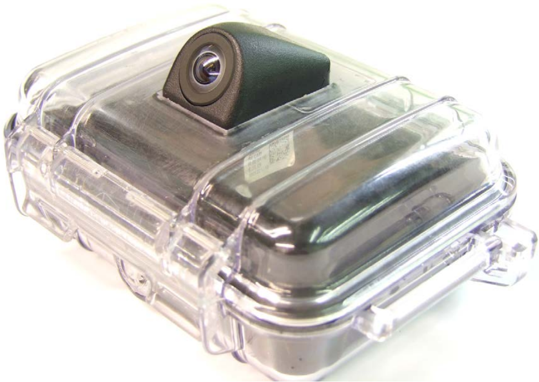
Figure 23 – Sample plastic environmental enclosure with camera installed.
