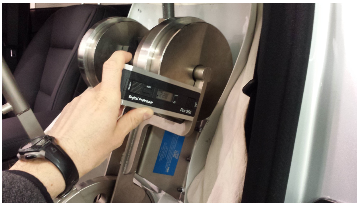
Figure 12 - Measurement of the H-point manikin machine torso weight hanger angle at 22.8 degrees. Adjust to 25 degrees from vertical.
