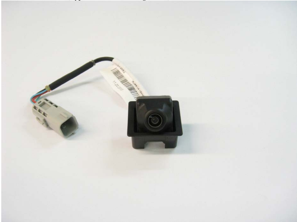
Figure 22 – Typical camera and associated connector and wiring removed from vehicle.
