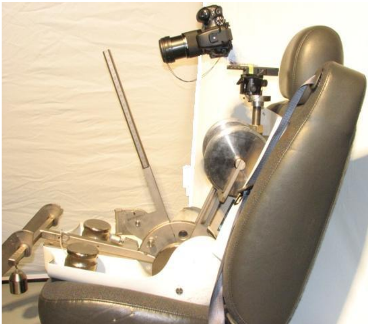
Figure 19 – Camera & Mounting fixture on Neck of H-Point Machine
