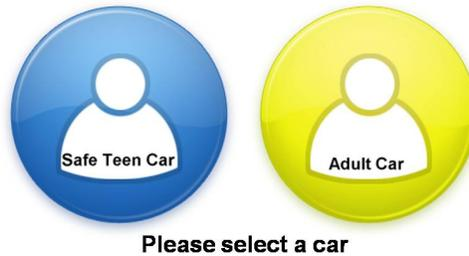
**Figure 5. Example Teen Driver Identification subsystem in-vehicle display to indicate a choice between Safer Teen Car and Adult Car modes.**
