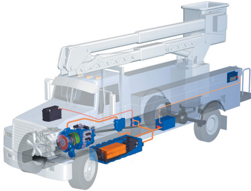
Figure 2-7: Schematic of a Parallel Hybrid-Electric Utility Truck 166
