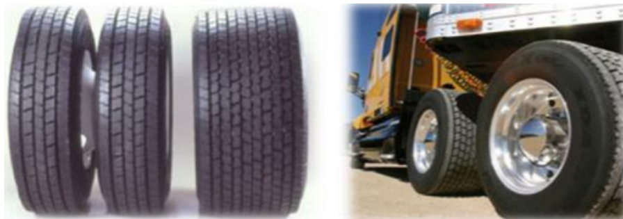
Figure 2-11: Single Wide Base Tires Replacing Duals at Each Wheel Site 309
