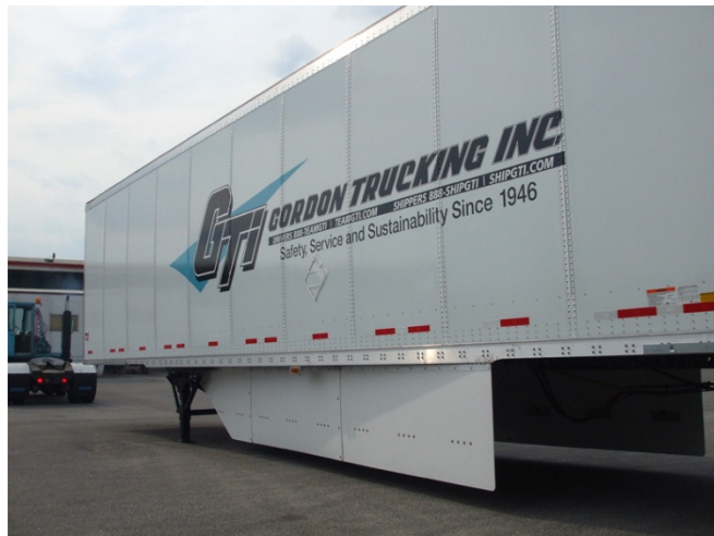
Figure 4-5: Trailer Skirt Made From Resilient Composite Material 451
