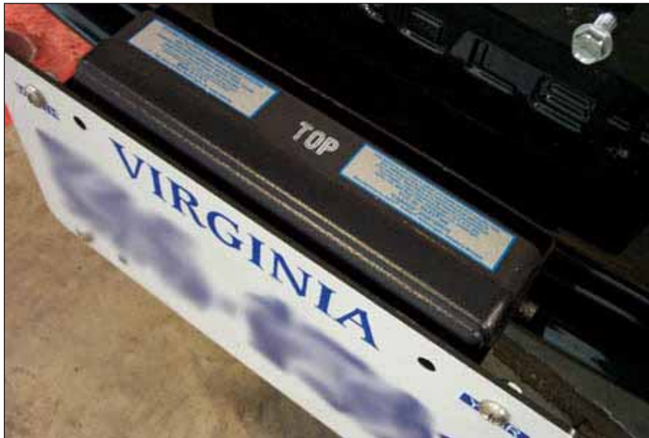
Figure 5. Doppler Radar Antenna Mounted on the Front of a Vehicle, Covered by one of the Plastic License Plates used for this Study
