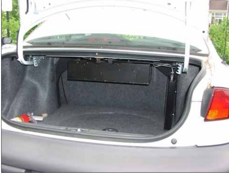
Figure 4. The Main DAS Unit Mounted under the “Package Shelf” of the Trunk
