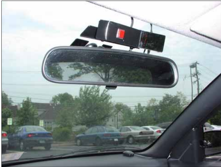
Figure 6. The Incident Pushbutton Box Mounted above the Rearview Mirror (The portion on the right contains the camera aimed at the driver’s face hidden by a smoked Plexiglas cover.)
