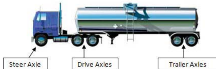
Figure 1-21 Class 8 Standard "18 Wheeler" Axle Identification
