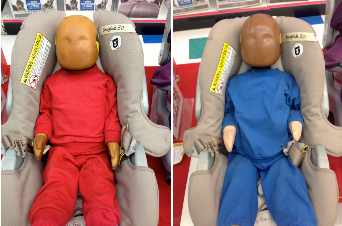
Figure 2. A single CRS model that provides good fit with the CRABI-12 (left) and tight fit with reduced head-to-CRS shell clearance with the CRABI-18 (right).
