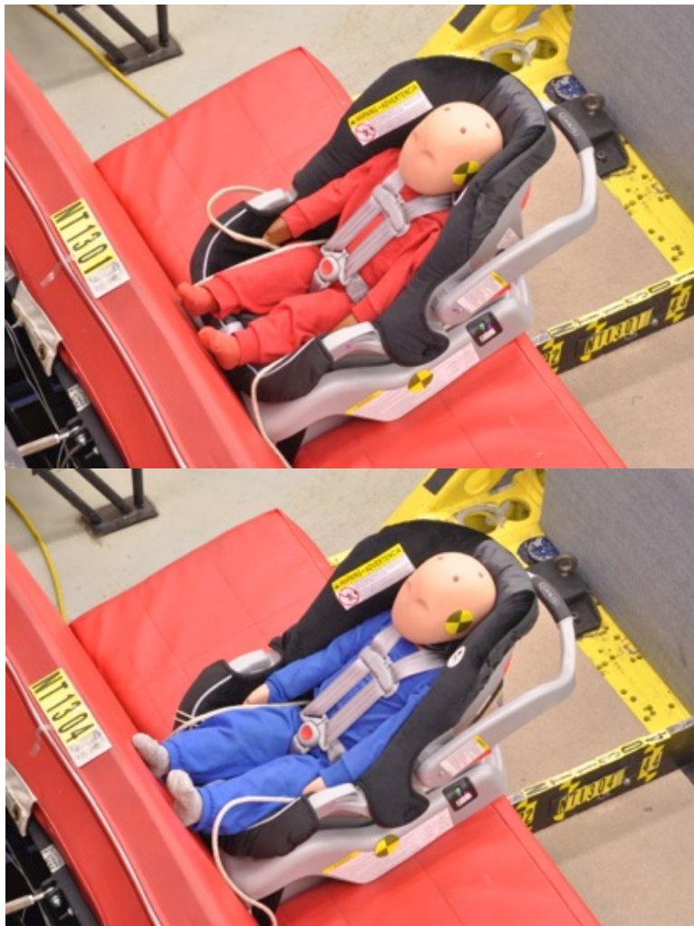
Figure 3. Pre-test photos of the Graco SnugRide 30 with the CRABI-12 (top) and CRABI-18 (bottom)
