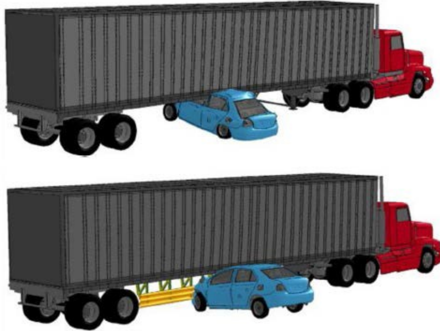
Figure 1.3 Computer finite element representation of the impact of a passenger vehicle into the side of a tractor-trailer without SUPD (top) and with SUPD (bottom) (Galipeau-Belair, Ghantae, Critchley, Ramachandra, & El-Gindy, 2014).
