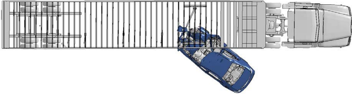
Figure 7.4 Passenger car underneath the trailer after impacting the landing gear region while traveling toward the rear of the tractor-trailer.
