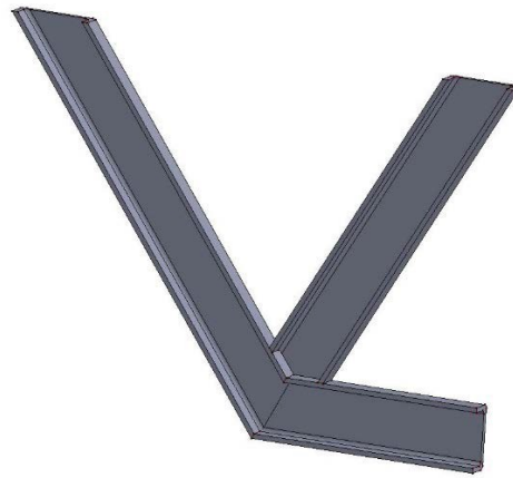
Figure 4.8 Brace design with diagonally oriented front member
