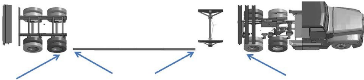
Figure 7.1 Four impact points shown for the gap impact evaluation. Various parts of the model are not shown to highlight the relative locations of the SUPD rail, landing gear, and rear tandem bogie.
