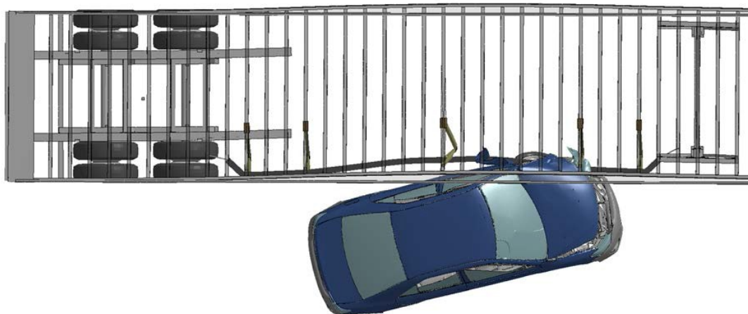
Figure 5.18 Top view of steel SUPD system with 3ft - 7ft - 7ft - 3ft brace spacing for 50-mph and 30-degree impact condition
