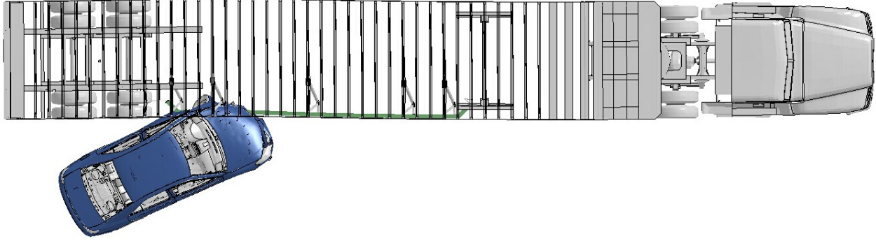
Figure 7.6 Passenger car impact with the tractor-trailer in the rear tandem region while traveling toward the front of the tractor-trailer
