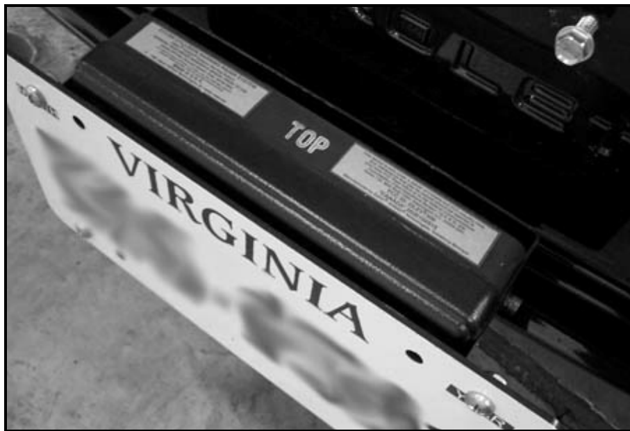
Figure 5. Doppler Radar Antenna Mounted on the Front of a Vehicle
