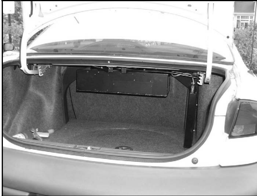
Figure 4. The Main DAS Unit Mounted Under the “Package Shelf” of the Trunk
