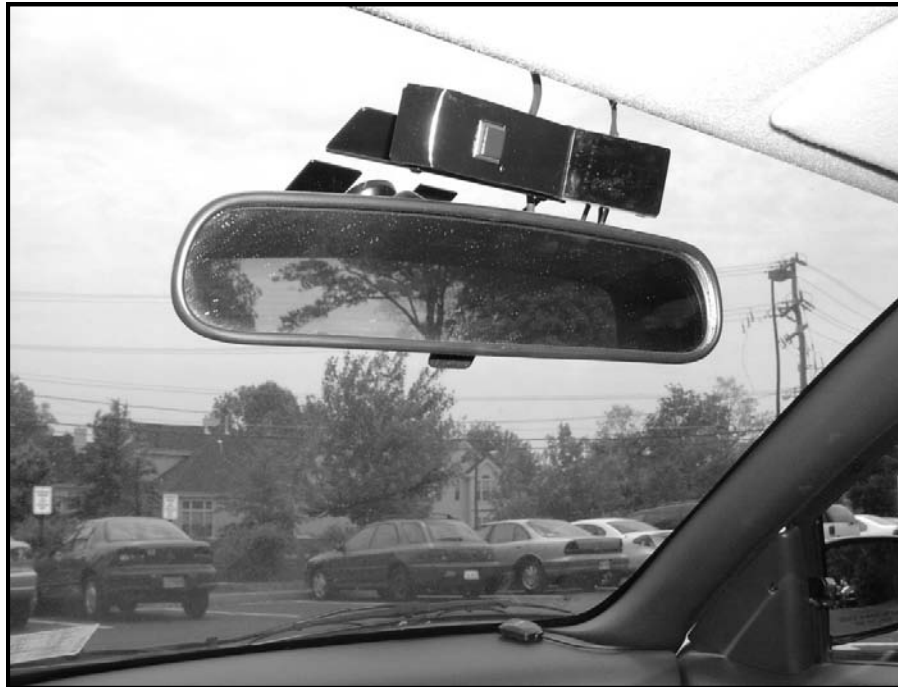
Figure 6. The Incident Pushbutton and Camera Box Mounted Above the Rearview Mirror
