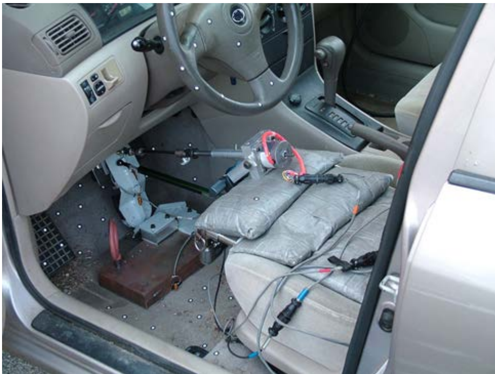
Figure 3 - Pedal Force and Displacement Measuring Device
