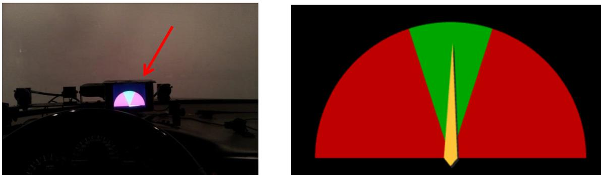
**Figure 13. Revised headway display location and configuration**
