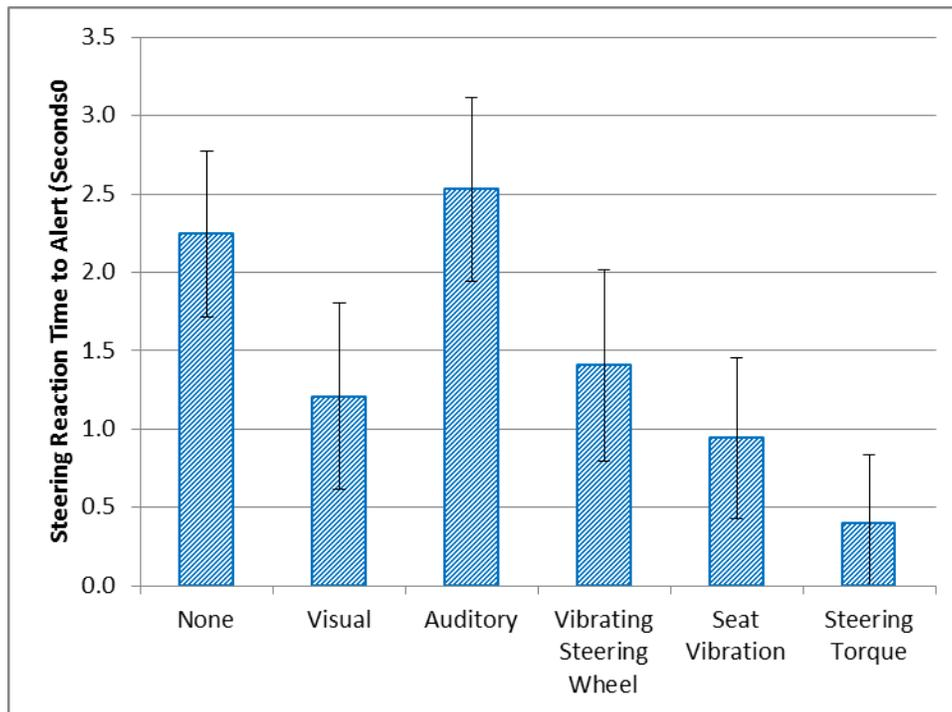
Figure 32. Effect of warning type on steering reaction time for the LDW false alarm event
