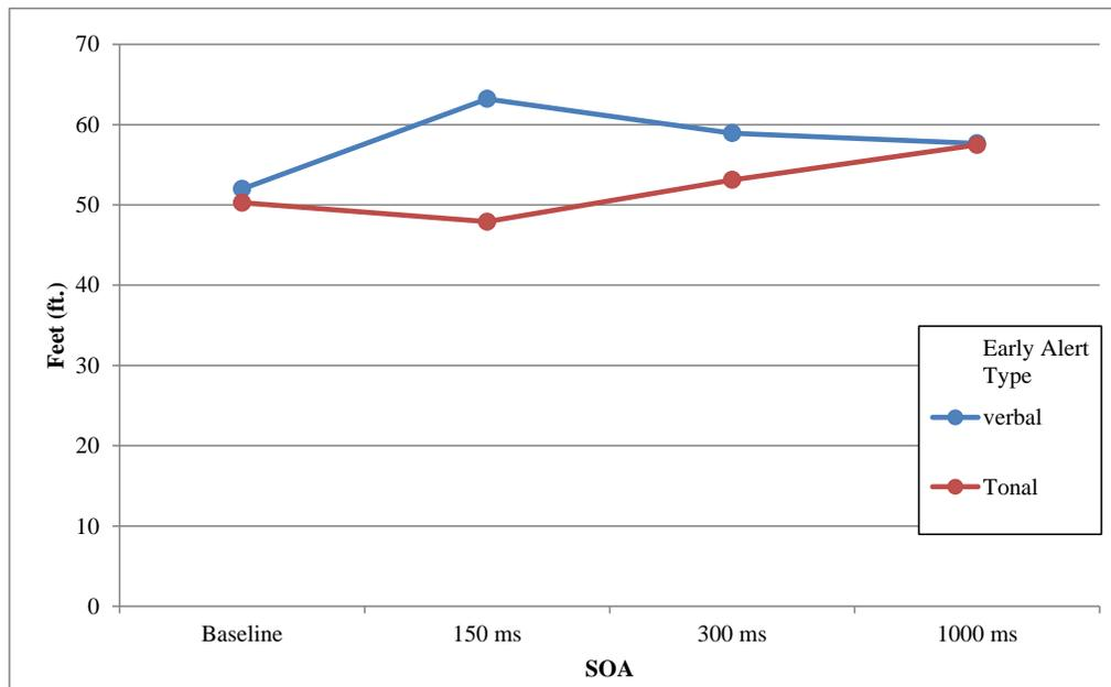
**Figure 60. Minimum distance between subject vehicle and lead vehicle as a function of early alert type and SOA (undistracted drivers)**
