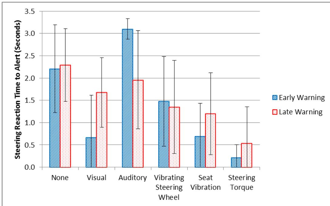
Figure 31. Effect of warning type and timing on steering reaction time for false alarm
