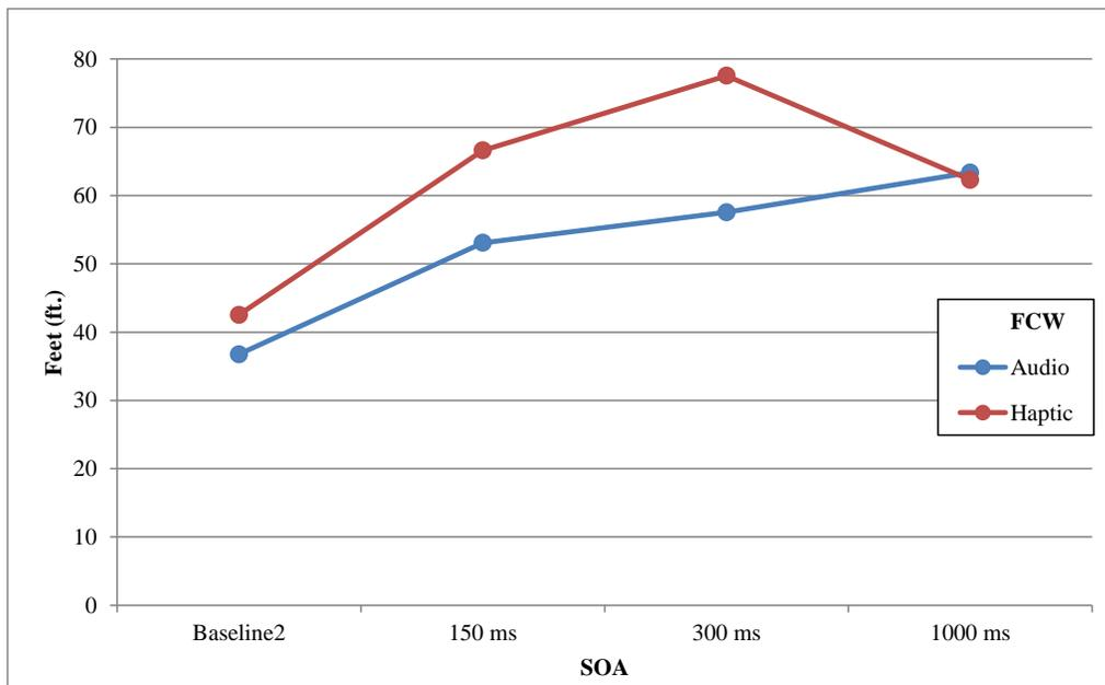
**Figure 64. Minimum distance between subject vehicle and lead vehicle as a function of FCW modality and SOA (distracted drivers)**
