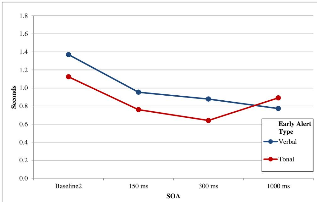
**Figure 61. Total response time as a function of early alert type and SOA (distracted drivers)**
