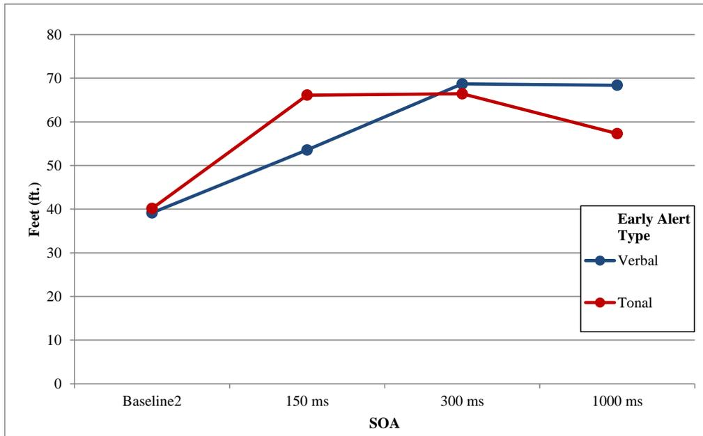
**Figure 63. Minimum distance between subject vehicle and lead vehicle as a function of early alert type and SOA (distracted drivers)**
