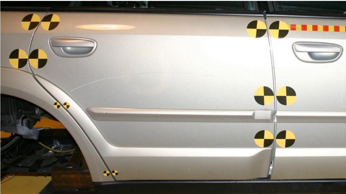
Figure 3. Typical Target Locations for Hinged Side Doors
