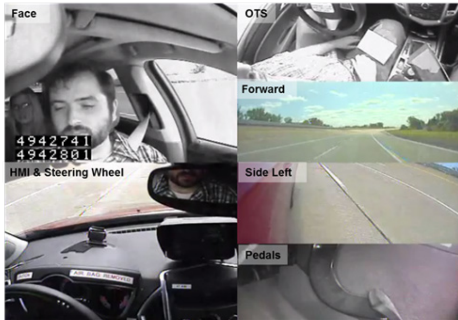
Figure 3-3. VTTI's DAS Camera Views for Experiment 2
