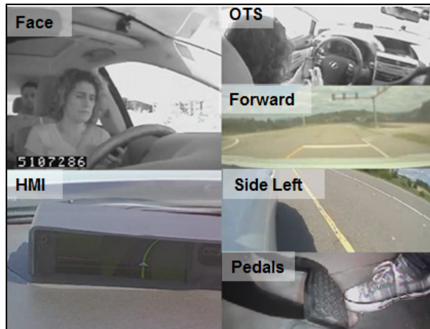
Figure 4-4. VTTI's DAS Camera Views from Experiment 3
