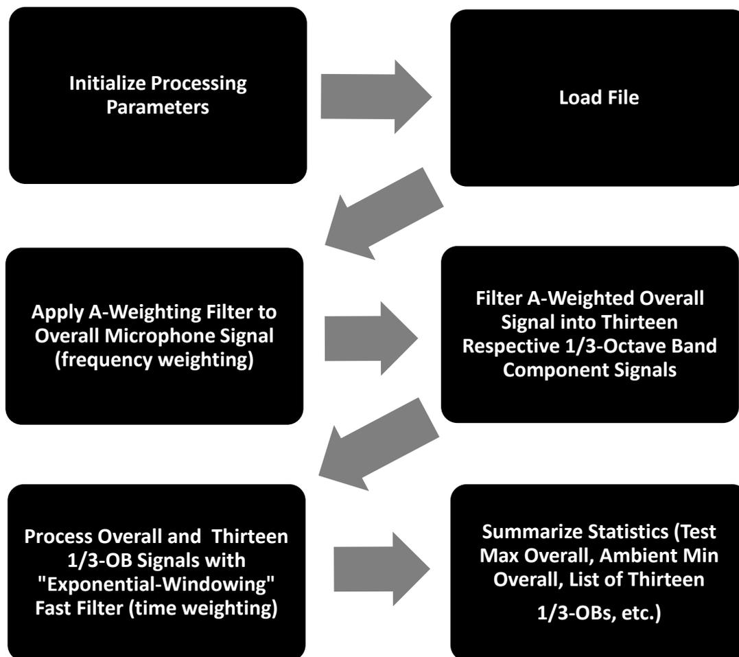
**Figure 13. General Flow Diagram for Data Processing Code**
