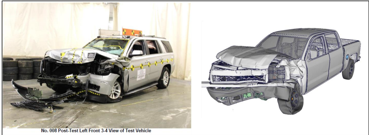
Figure 76: NHTSA Oblique Impact Post-Crash – 2016 Tahoe Versus CAE Baseline
