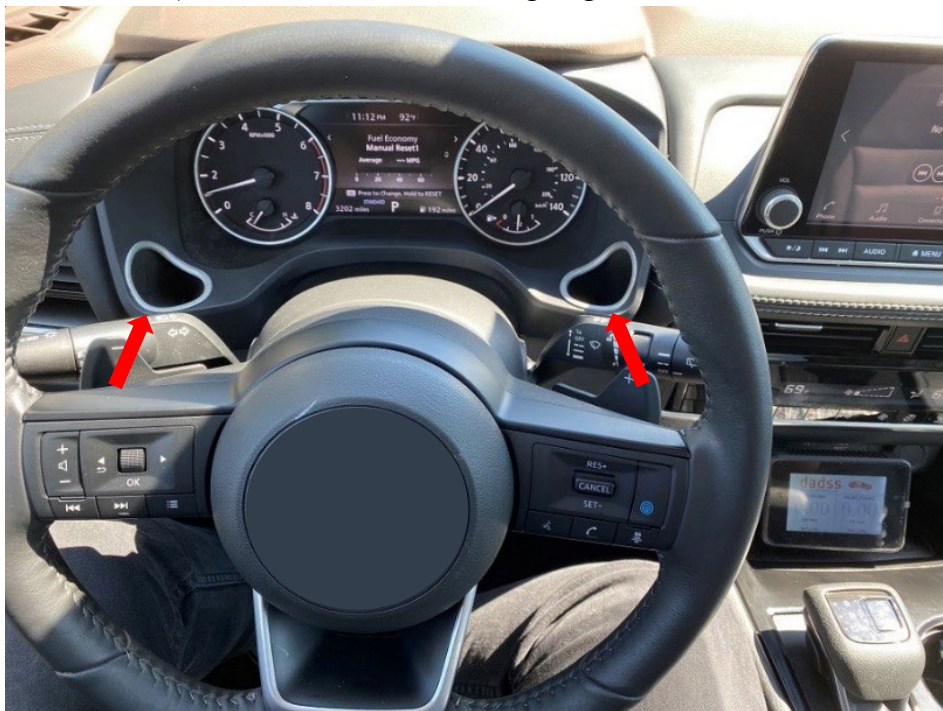
Figure 34. Compact SUV with newly designed inlets in the instrument cluster
