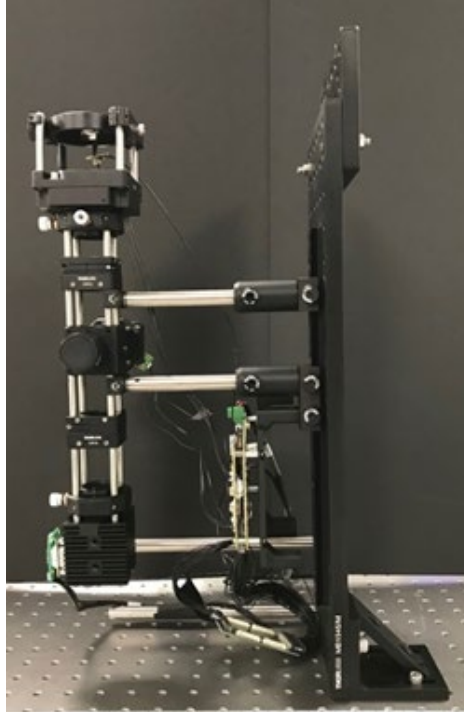
Figure 15. Vertical benchtop reflectance system
