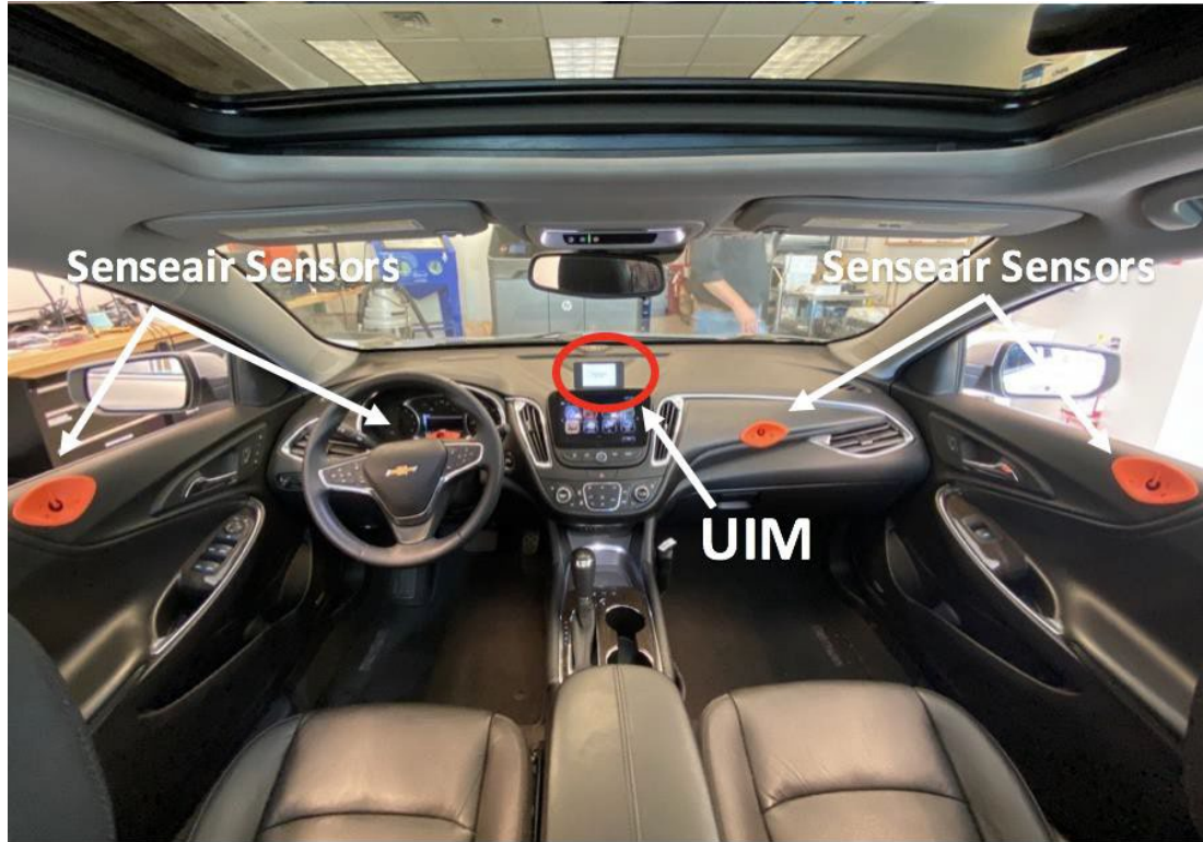
Figure 30. Position of the breath sensors on the driver (left) and passenger sides of the vehicle and user interface module (UIM)
