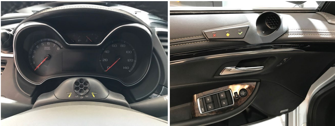
Figure 1. Third Generation breath-based sensor integrated into DADSS X2 research vehicle steering column (left) and driver door panel (right)
