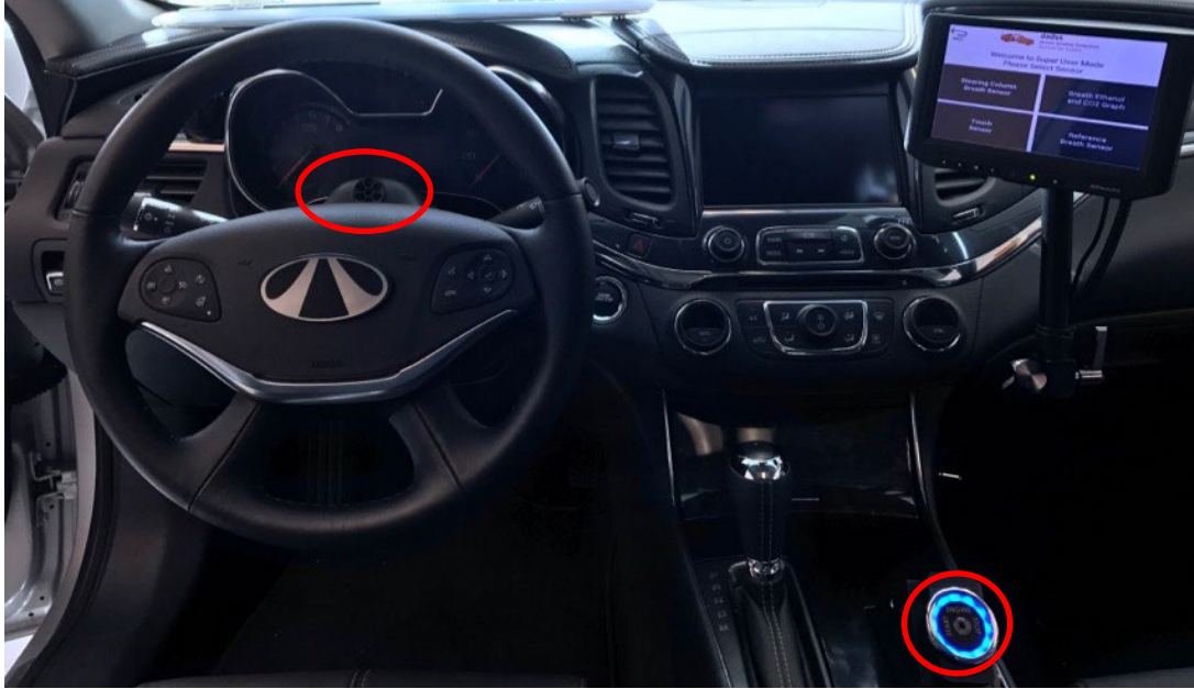
Figure 6. DADSS X2 interior with steering column breath-based sensor (top left), touch-based sensor (bottom right), and control monitor (top right)
