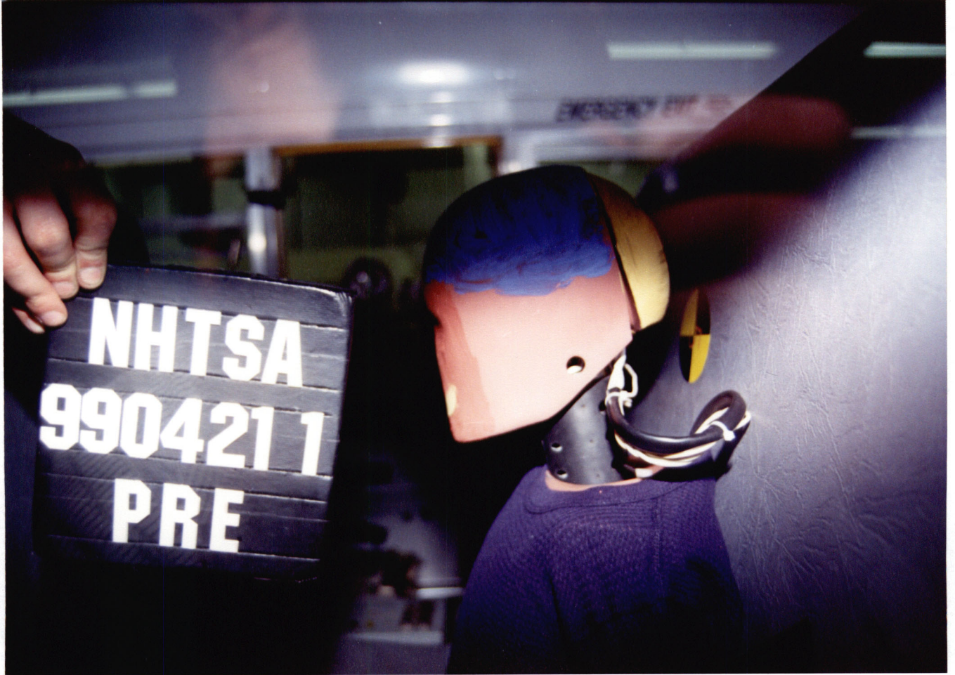
Figure A-21 Pre-Test Left Side Seat 4 Instrumented 6 Year Old - View 1
