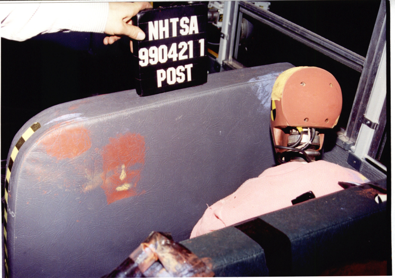
Figure A-52 Post-Test Right Side Seat 6 Instrumented 5 th and 6 Year Old - View 5
