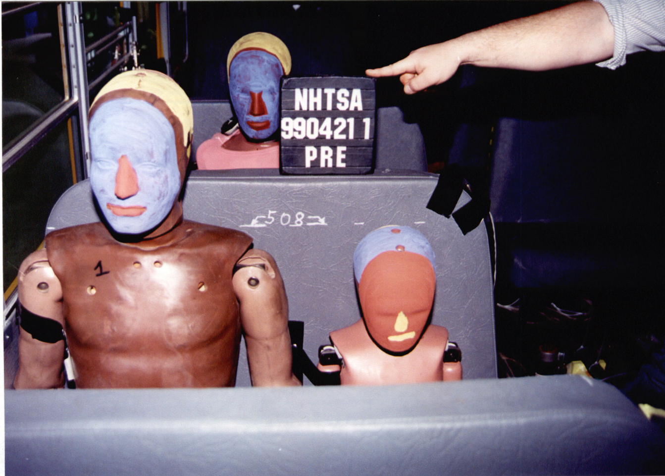
Figure A-17 Pre-Test Right Side Seat 1 Ballast 50 th and 6 Year Old - View 3
