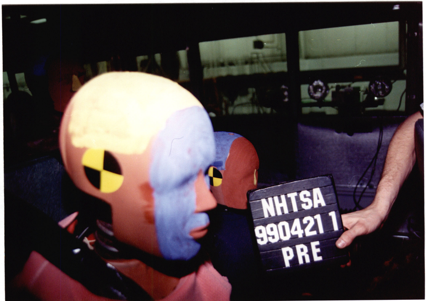
Figure A-24 Pre-Test Right Side Seat 6 Instrumented 5 th and 6 Year Old - View 1
