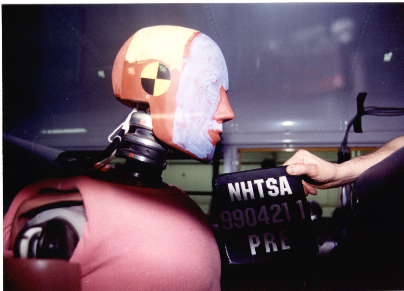
Figure A-18 Pre-Test Right Side Seat 2 Instrumented 50 th - View 1
