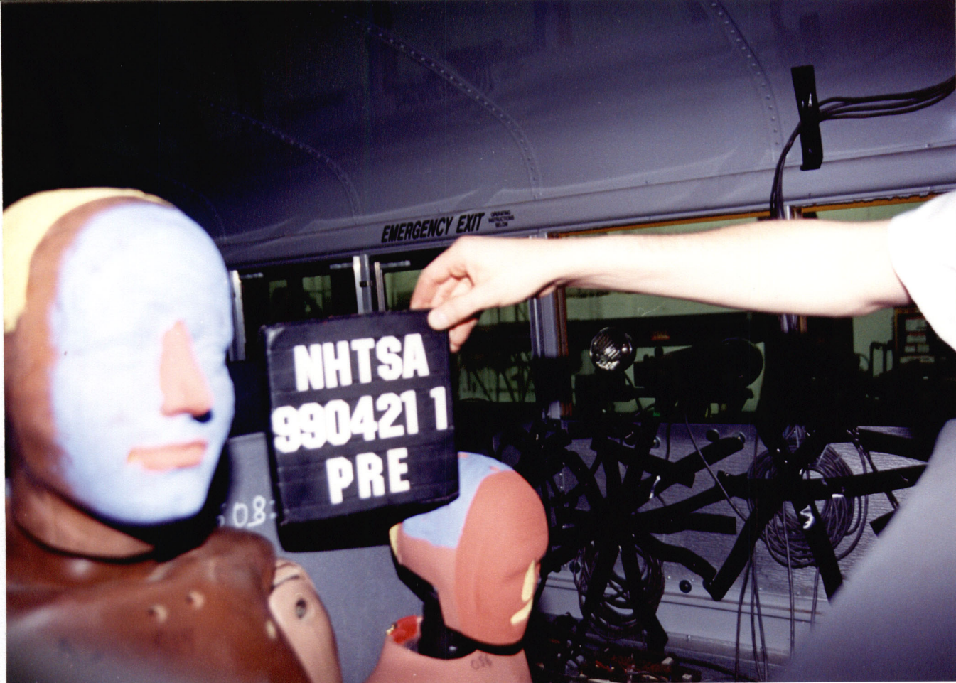
Figure A-15 Pre-Test Right Side Seat 1 Ballast 50 th and 6 Year Old - View 1
