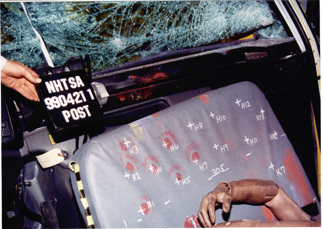
Figure A-38 Post-Test Right Side Seat 1 50 th and 6 Year Old Ballast - View 3
