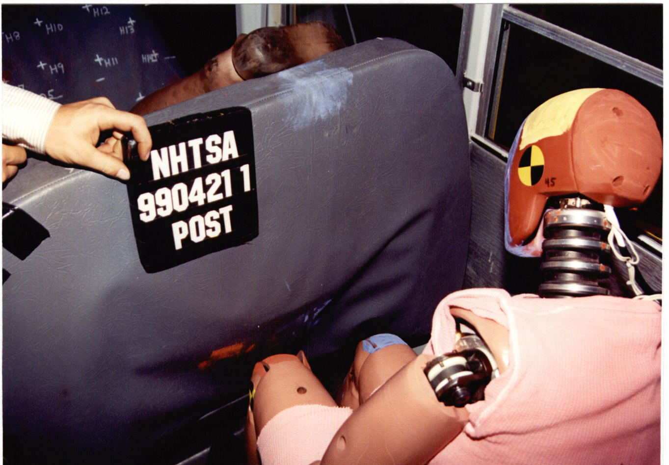
Figure A-41 Post-Test Right Side Seat 2 Instrumented 50 th - View 1
