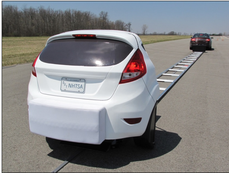
Figure 2-3 NHTSA's Strikeable Surrogate Vehicle (SSV)
