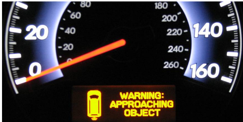
Figure 7. Photo of Warning Message from Odyssey Parking Sensor System
