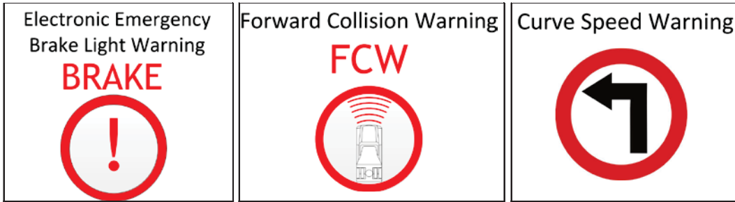
Figure 19: CS-SwRI RSD HMI Visual Warning Messages (EEBL, FCW, and Left CSW)
