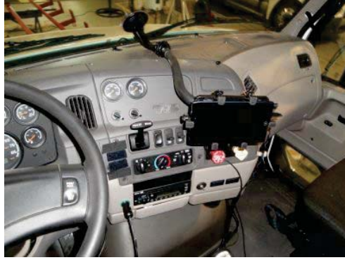
Figure 13: CS-SwRI Retrofit Installation in Conway Truck
