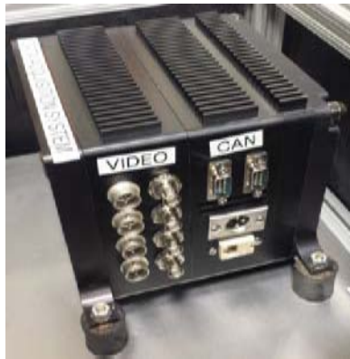
Figure 21: SwRI Data Acquisition System
