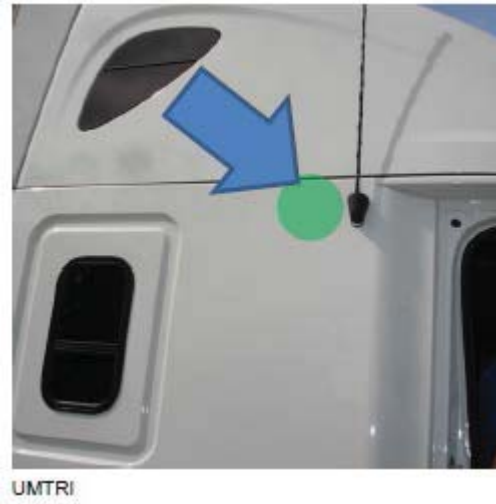
Figure 2: Illustration of DSRC Antenna on Integrated Truck
