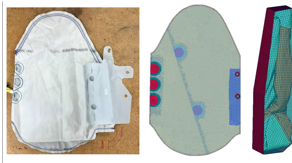
Figure 35: Side Air Bag FE Model Before and After Folding
