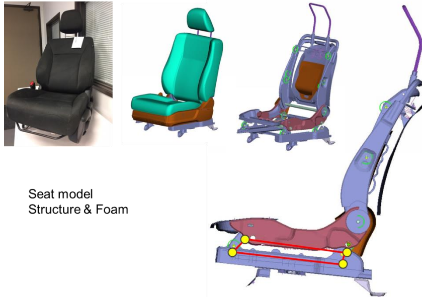
Figure 25: Seat FEM – Height Adjustment Mechanism
