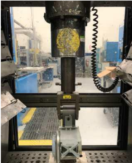
Figure 43: Retractor Pay-out (load limiter) Test Setup
