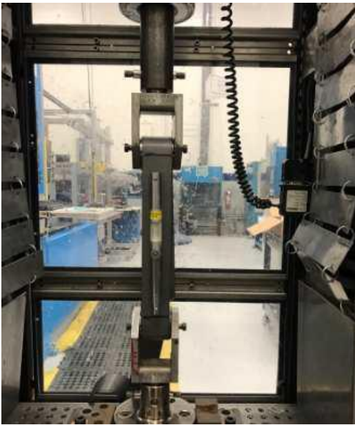
Figure 42: Webbing Elongation Test Setup
