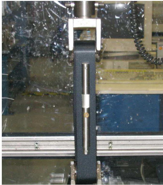
Figure 42: Webbing Elongation Test Setup
