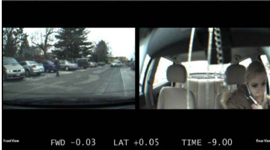
Figure 2. Exterior and interior video view captured by cameras on the DriveCam event recorder (image provided by DriveCam)
