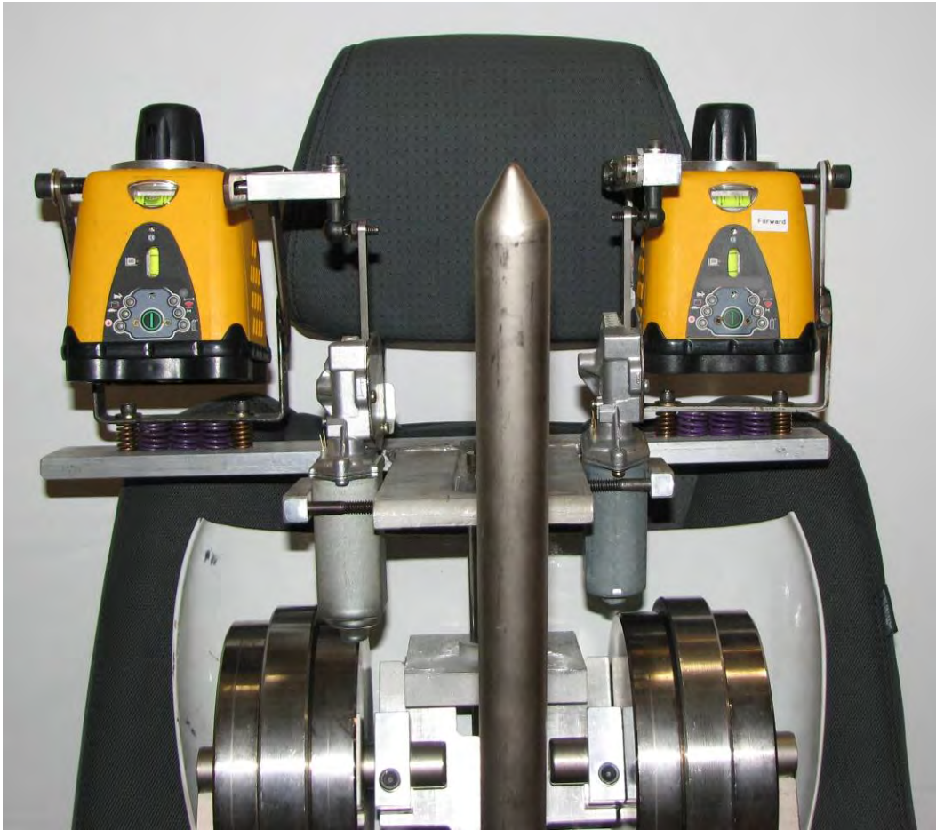
Figure 3. Rear-Looking laser Fixture Used to Simulate the Line of Sight of a 50th Percentile Male Driver.
