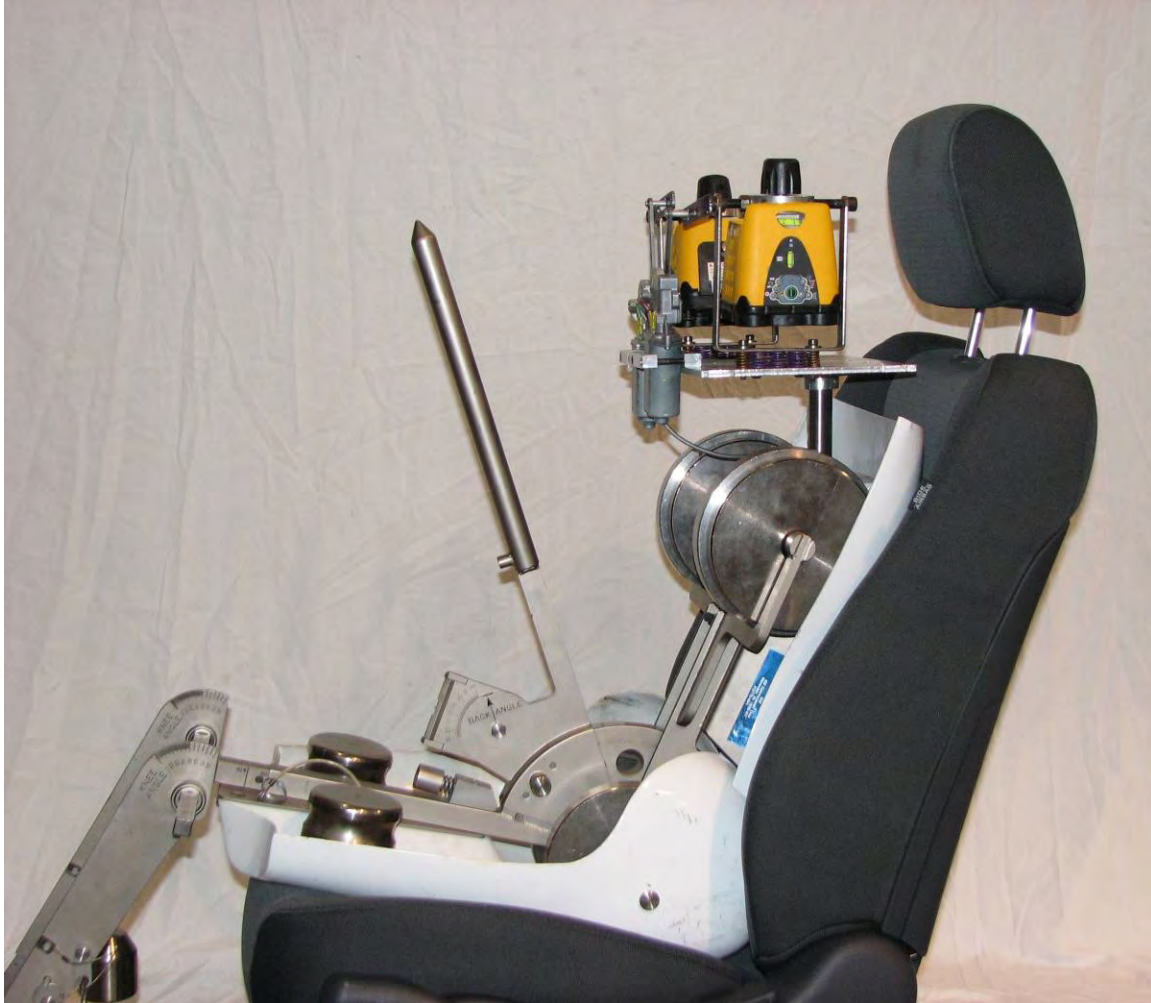
Figure 4. Side view of Side-Looking laser Fixture Used to Simulate the Line of Sight of a 50th Percentile Male Driver.
