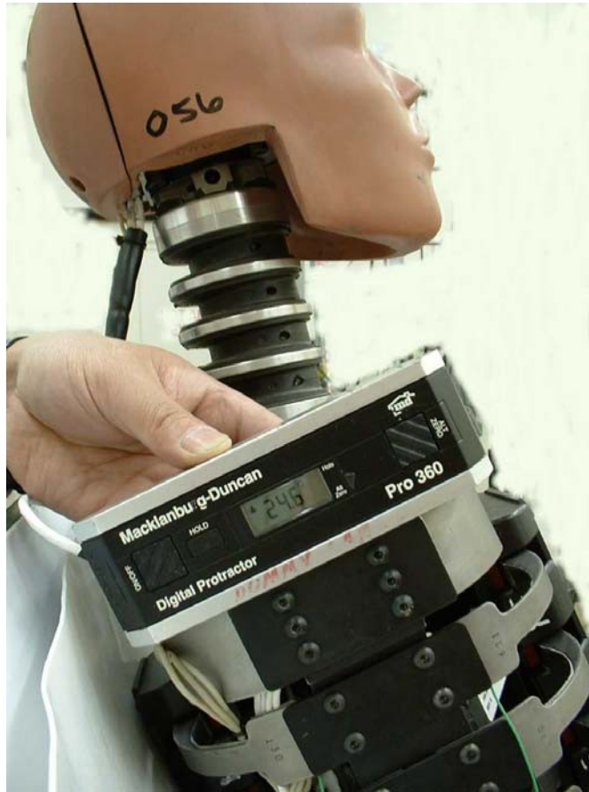
Figure 60. Adjusting the SID-II s D in the fore/aft plane for pelvis acetabulum test
