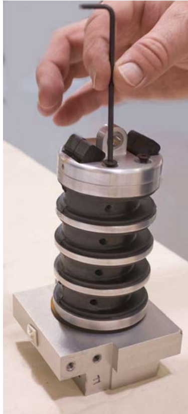
Figure 22. Reinstall neck nodding joint assembly
