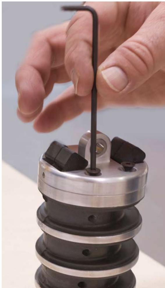
Figure 17. Removing the nodding joint assembly
