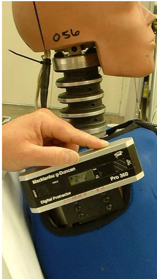
Figure 46. Adjusting the SID-II s D in the fore/aft plane
