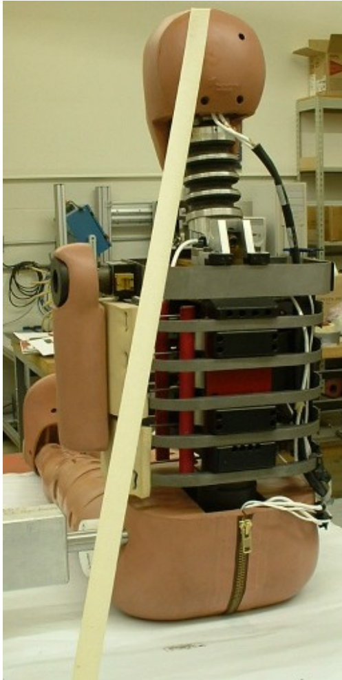
Figure 62. Using masking tape to seat the dummy upright
