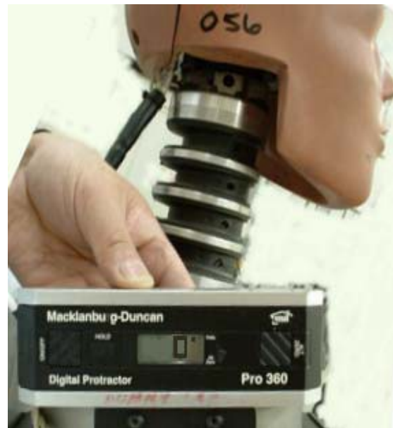
Figure 63. Adjusting the SID-IIsD in the fore/aft plane for pelvis iliac test
