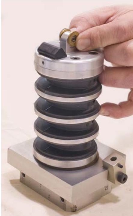
Figure 24. Install brass nodding joint washers
