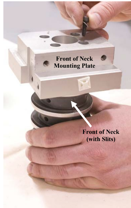
Figure 19. Assemble molded neck to neck mounting plate
