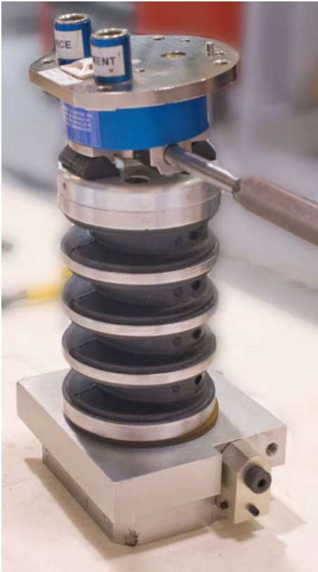
Figure 26. Align brass nodding joint washers with holes
