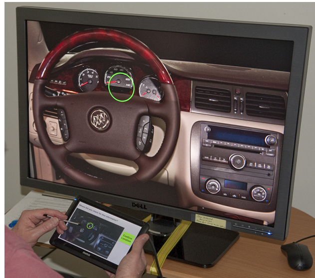
Figure 12. Participant using stylus to indicate information location on touch pad
