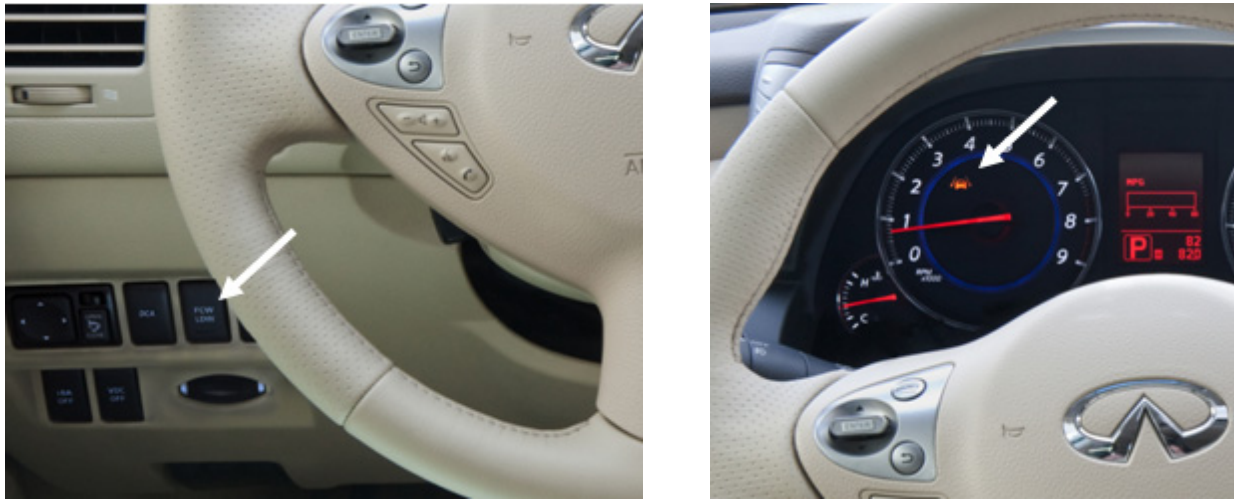
Figure 13. Infiniti LDW control button (left) and orange status indicator icon (right)
