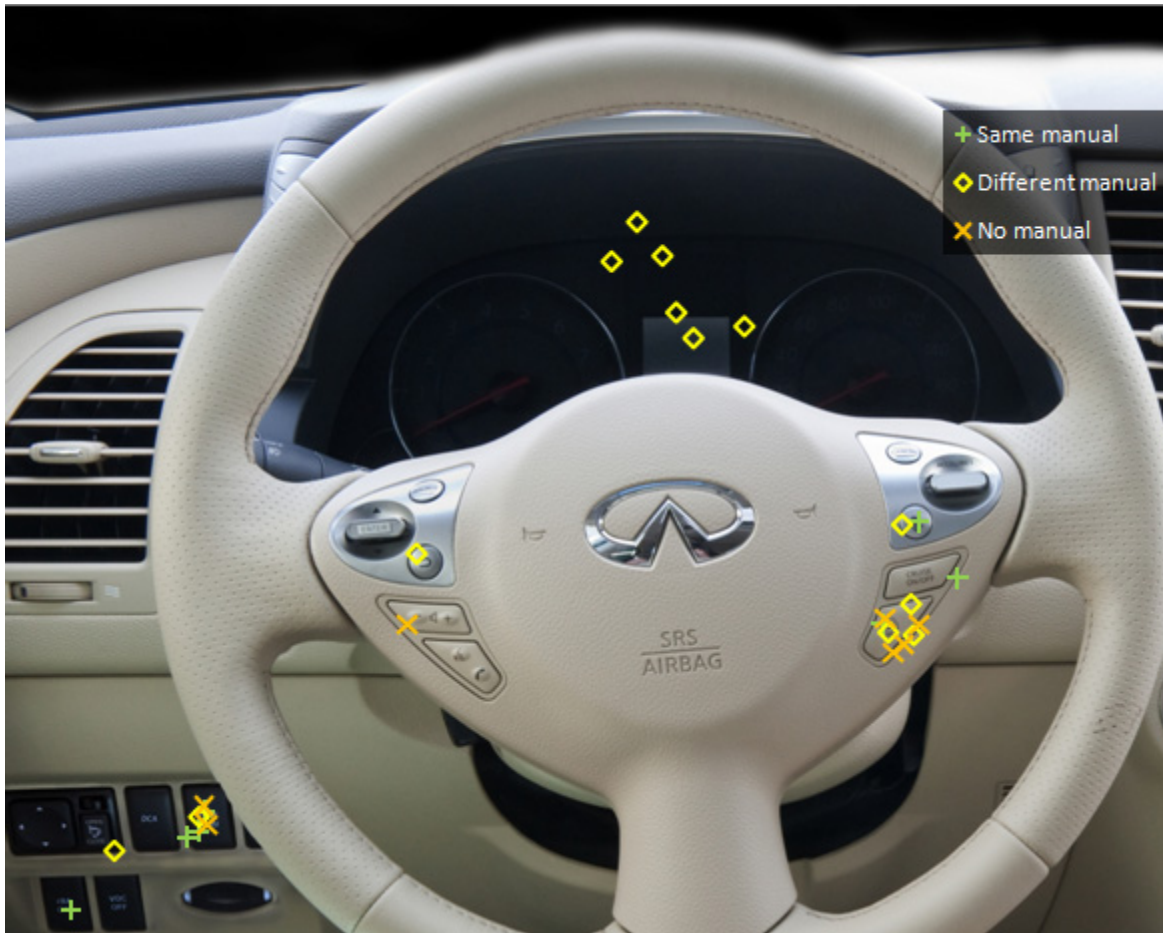
Figure 17. Pre-startup Infiniti example showing where participants looked to determine LDW system presence
