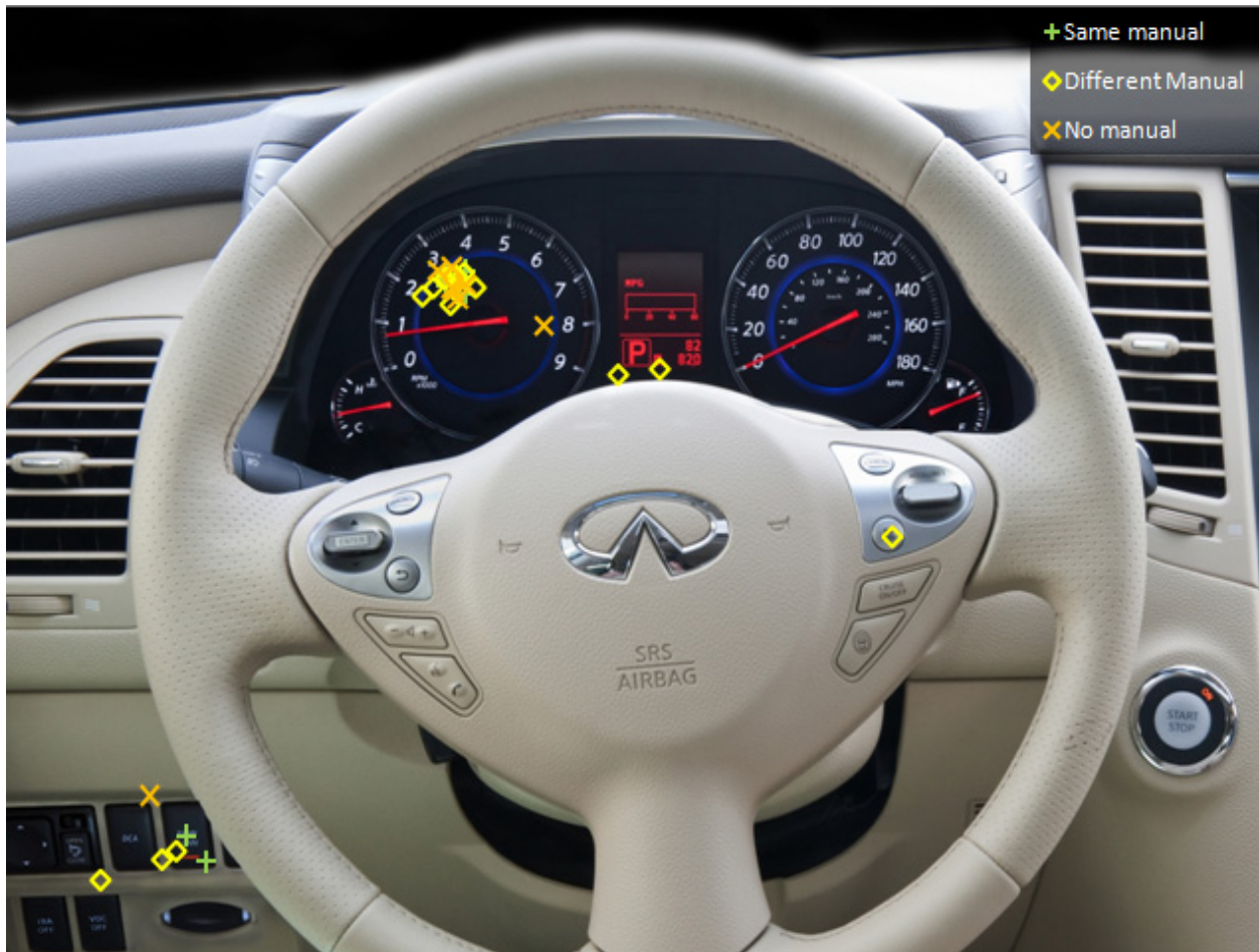
Figure 20. Image showing where participants clicked to indicate where they found information about LDW functionality, with most clicks clustered on orange LDW icon in speedometer
