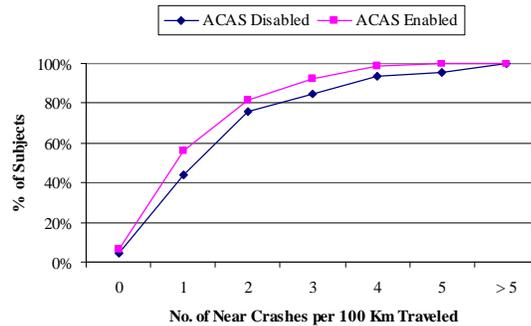
**Figure D-72. Distribution of High-Intensity Near-Crashes, ACAS Vehicle Speed >35 mph, ACAS-Disabled versus ACAS-Enabled**
