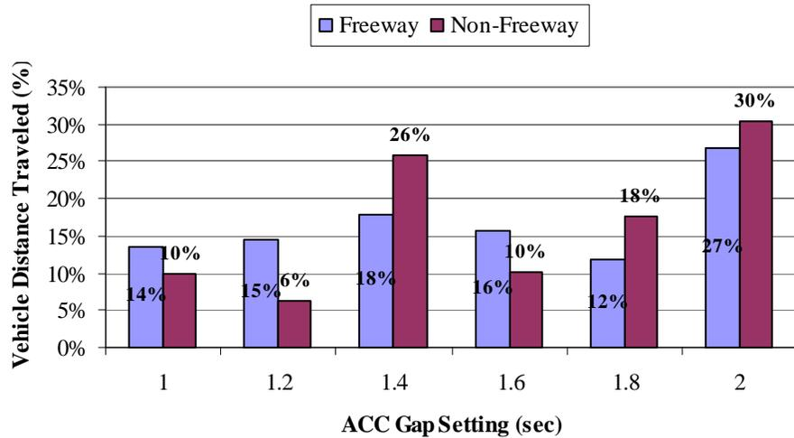
**Figure 2-48. Distribution of ACC Gap Settings by Road Type, Period 4**
