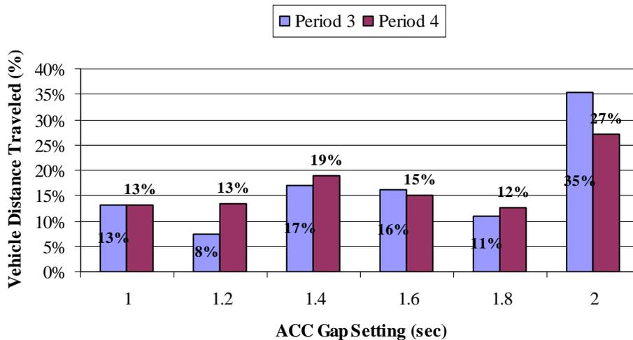
**Figure 2-46. Distribution of ACC Gap Settings, Period 3 versus Period 4**
