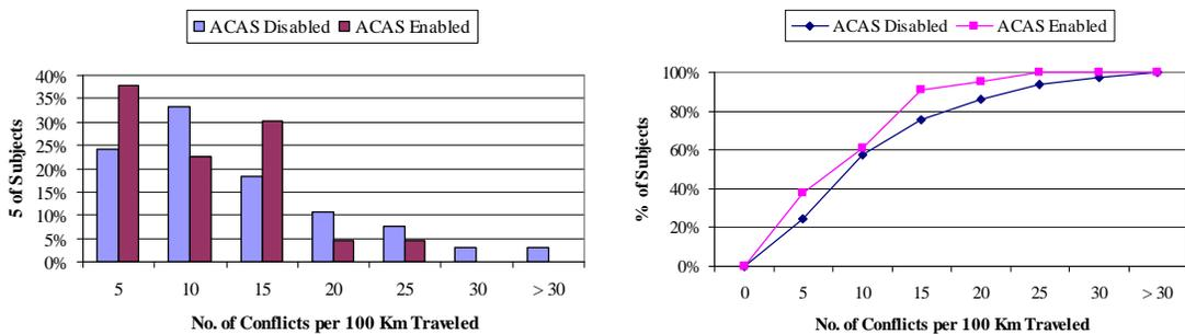
**Figure D-69. Distribution of Low-Intensity Conflicts, ACAS Vehicle Speed >35 mph, ACAS-Disabled versus ACAS-Enabled**
