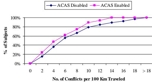
**Figure D-70. Distribution of High-Intensity Conflicts, ACAS Vehicle Speed >35 mph, ACAS-Disabled versus ACAS-Enabled**
