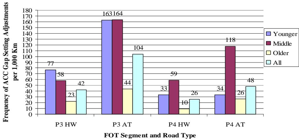
**Figure U-3. Frequency of ACC Gap Setting Changes by FOT Segment, Road Type, and Driver Age Group**
