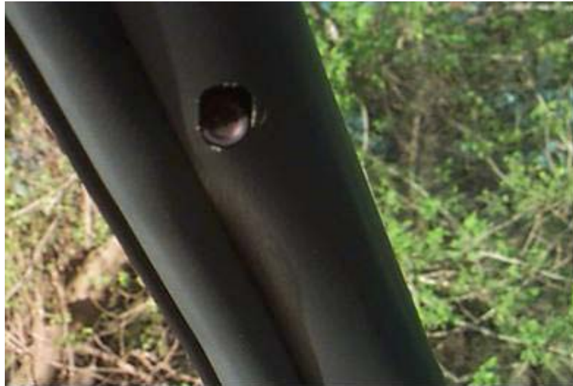
Figure 2.6. Driver's Face Camera Mounted in the A-pillar.
