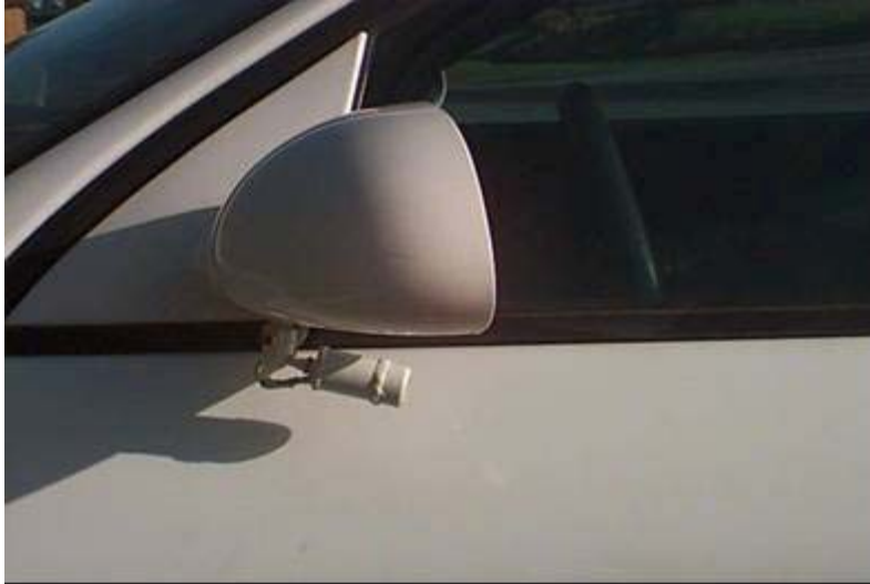
Figure 2.7. Camera Mounted Under the Side Mirror.
