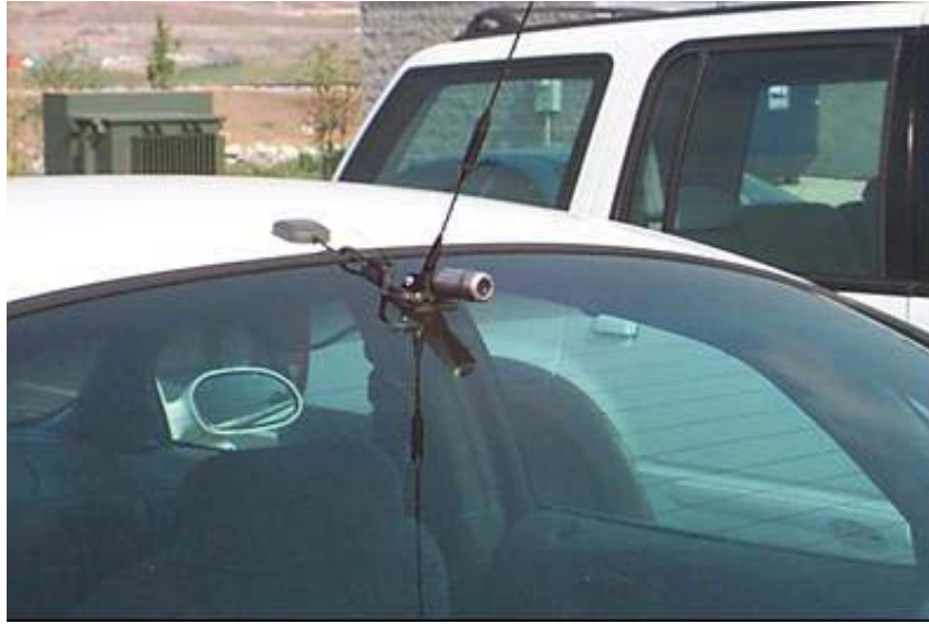
Figure 2.5. Rearview Video Camera above the Rear Window.
