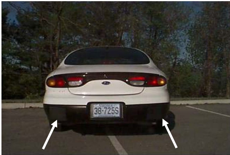
Figure 2.12. Rear Radar Units Embedded in Black Bumper.
