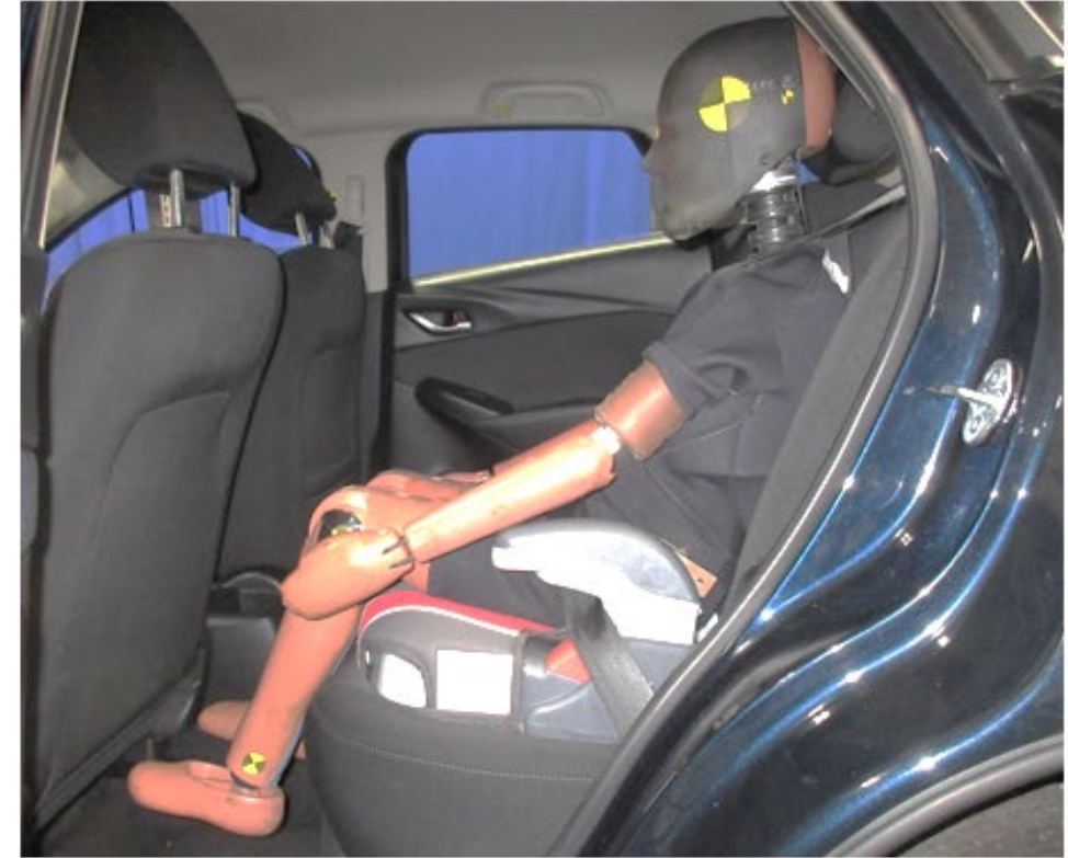
Mazda CX-3, LODC, CW_2, Passenger Seat, With Graco Turbo Booster, Hip Point set at 35°
