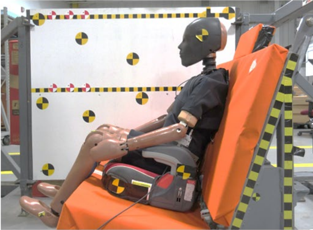
213 Bench, LODC, CW_2, With Graco Turbo Booster, Hip-Point set at 35°
