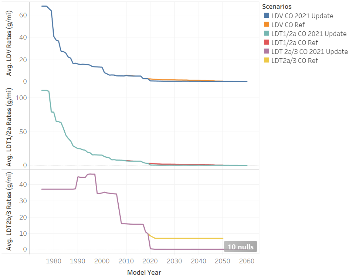
Figure 5-4 – Illustration of Newly Updated CO Emission Rate Projections for Gasoline Cars and Light Trucks Over the Next 40 Years
