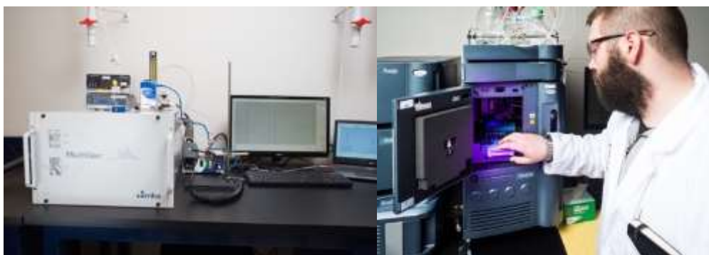
Figure 11. MKS Multigas 2030 FTIR for breath –based samples and Waters Acquity HPLC for touch-based samples in the DADSS Research Laboratory
