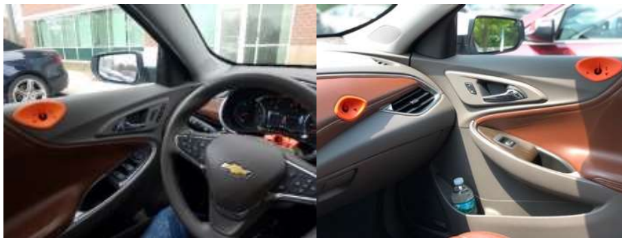
Figure 14. Position of the breath sensors on the driver (left) and passenger sides of the vehicle
