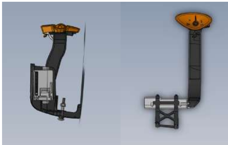
Figure 19. Design of breath sensor delivery systems (snorkels) from the breath inlet port to the sensor
