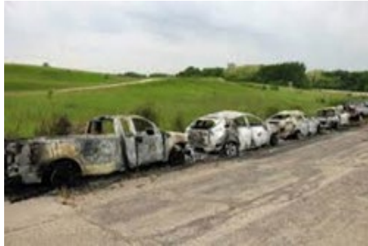
2011 Chevy Volt Latent Battery Fire at DOT/NHTSA Test Facility
