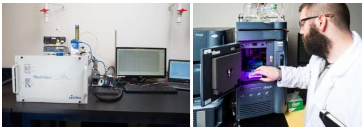
Figure 7. MKS Multi-gas 2030 FTIR for breath -based samples and Waters Aquity HPLC for touch-based samples in the DADSS Research Laboratory
