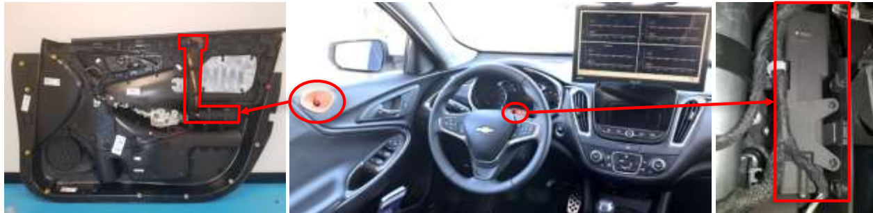
Figure 10. Platform development 2017 Chevrolet Malibu integrated with the breath-based sensors
