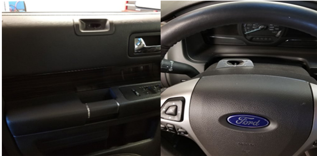
Figure 27. Sensor location in the driver door and at the top of the steering wheel.
