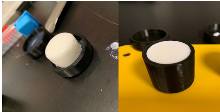
Figure 22. Tissue surrogates using 2% alginate gel (left) and 5% porcine gel (right)
