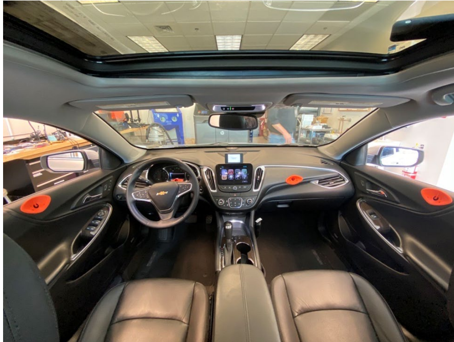
Figure 25. Position of the breath sensors on the driver (left) and passenger sides of the vehicle
