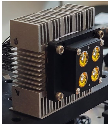
Figure 13. Back-end assembly (heatsink and lenses)
