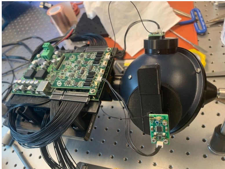
Figure 11. 3"integrating sphere/stingray lasers setup for measuring ethanol in transmission mode
