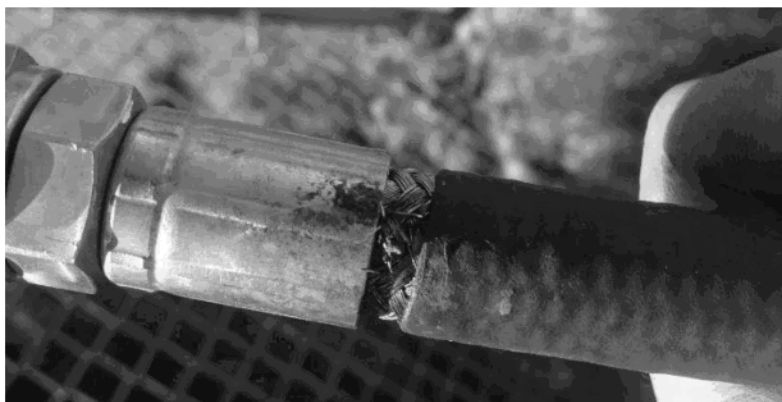
Figure 2 Corrosion on CNG hose braid and fitting.
