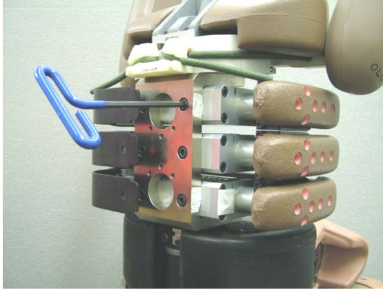
Figure 22. Removal of rib module
