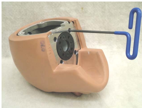
Figure 7. Removal of upper neck load cell structural replacement
