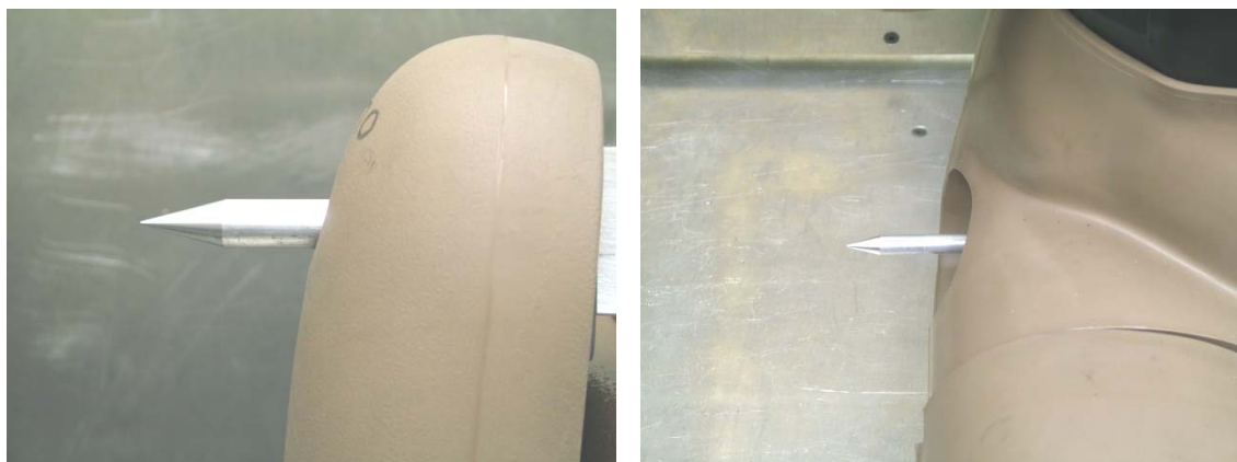
Figure 4. Threaded cylindrical tools installed at the shoulder and pelvis
