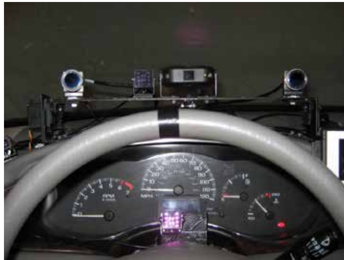
Figure 28 Eye and head tracking camera and infrared pod placement.
