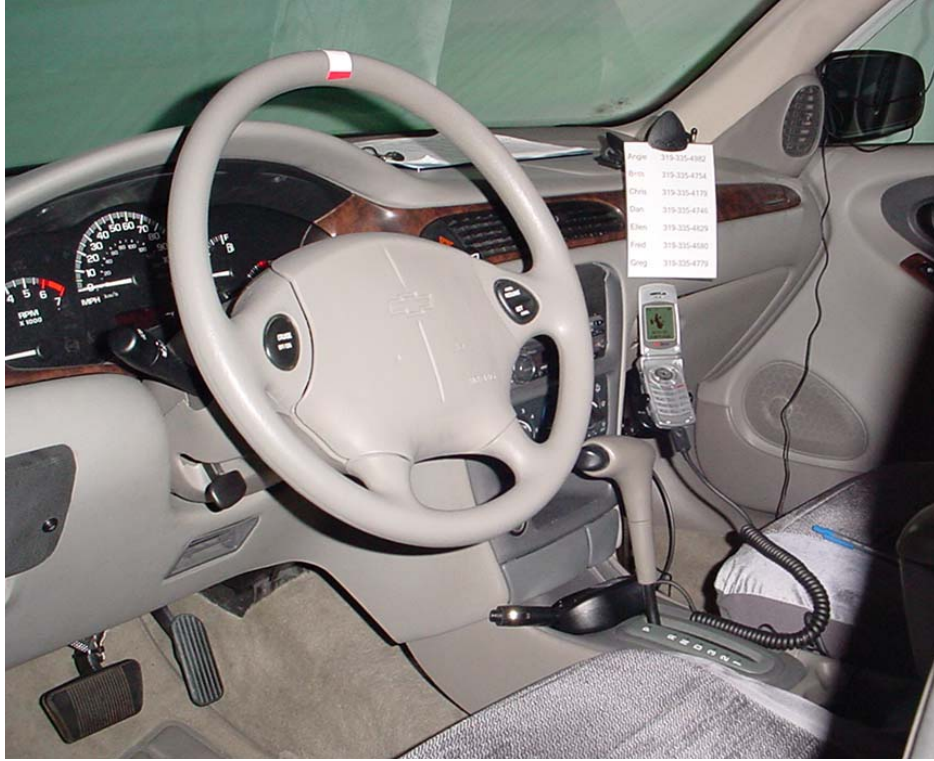
Figure 11. Photograph showing VSHF Hands-Free Speaker Kit setup and phone cradle location.
