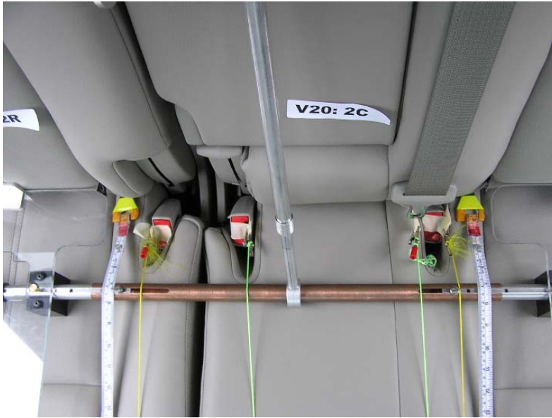
Figure 9. Most common arrangement of each pair of lower anchors between the outboard position seat belt anchors, and center seat belt anchors between the outboard buckle anchors.
