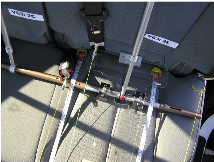
Figure 3. Example of anchor arrangement where LATCH belt and center seat belt webbing would have to cross if child restraints are installed in adjacent positions.
