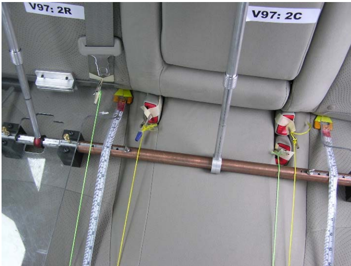
Figure 11. In the 2010 Toyota Prius, the center webbing is outboard of the right inboard lower anchor.
