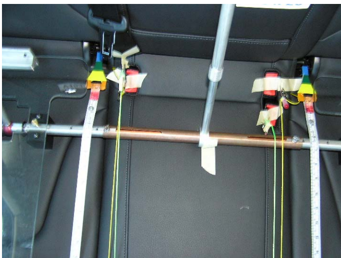
Figure 1. Example with at least 50 mm lateral spacing between lower anchors (attached to measuring tape) and nearby seat belt hardware (yellow and white strings), but less than 25 mm between seat belt hardware anchors for the outboard and center positions.
