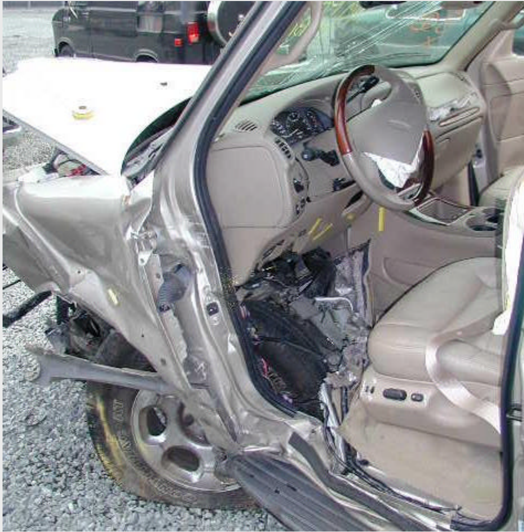
55 cm (21") longitudinal intrusion of toe pan
