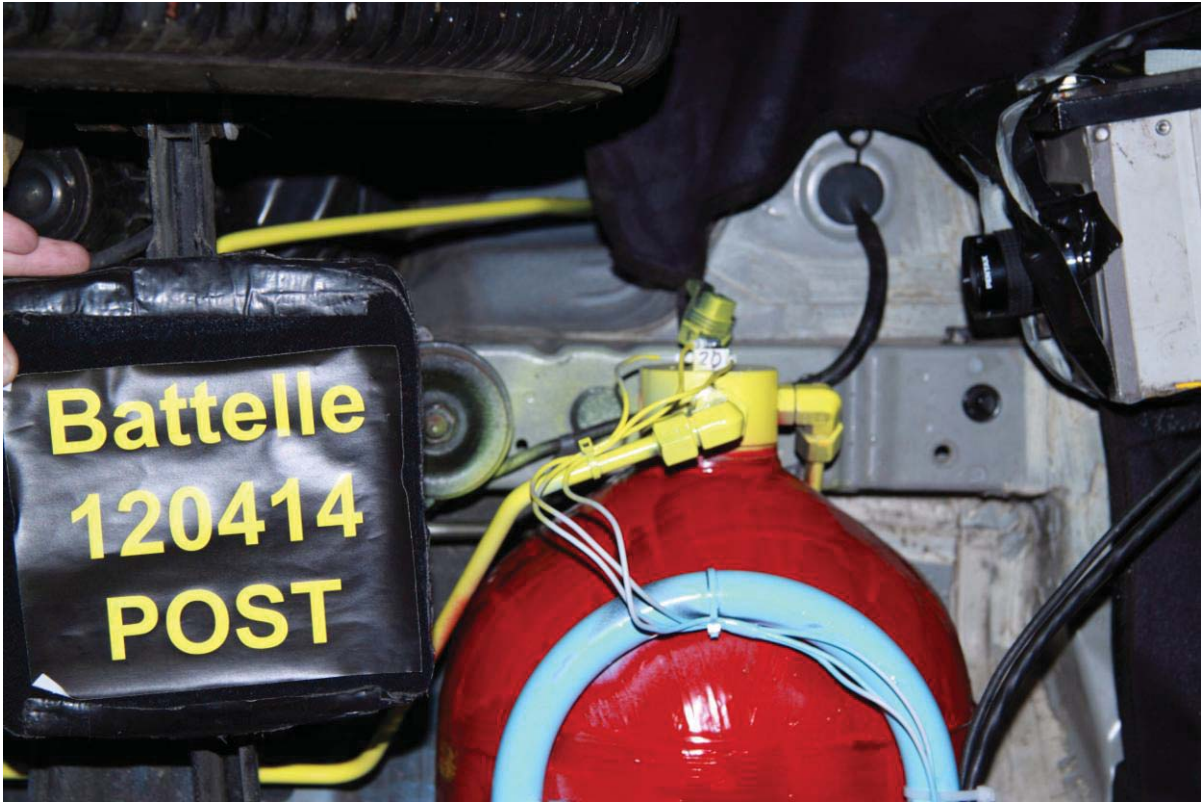
Figure A-37 Post-Test Fuel Lines - View 4
