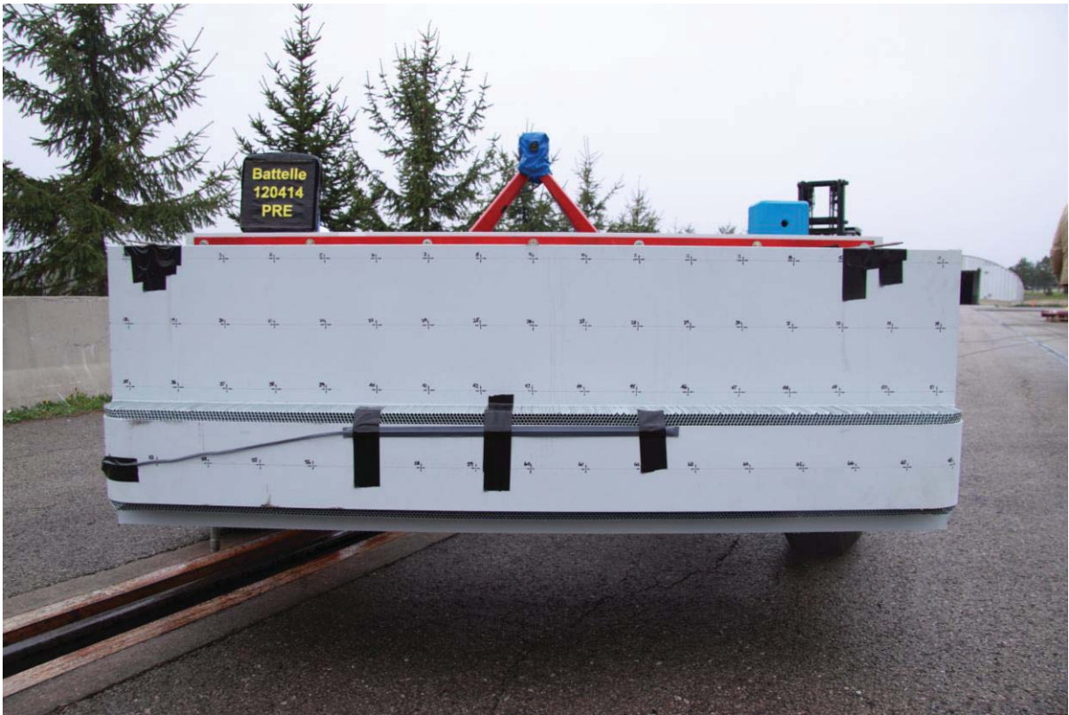
Figure A-51 Pre-Test Moving Barrier Front View
