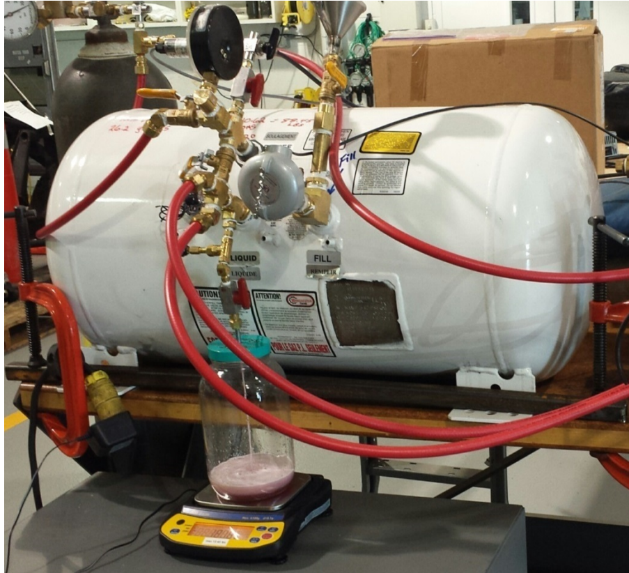
Figure 1 - Typical 26.2 Gallon LPG Automotive Fuel Tank with Test Components
