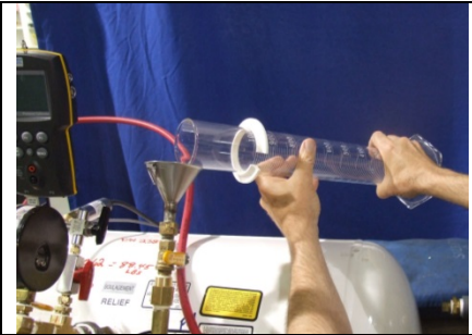
A. The tank is initially filled to 40 percent capacity with water
